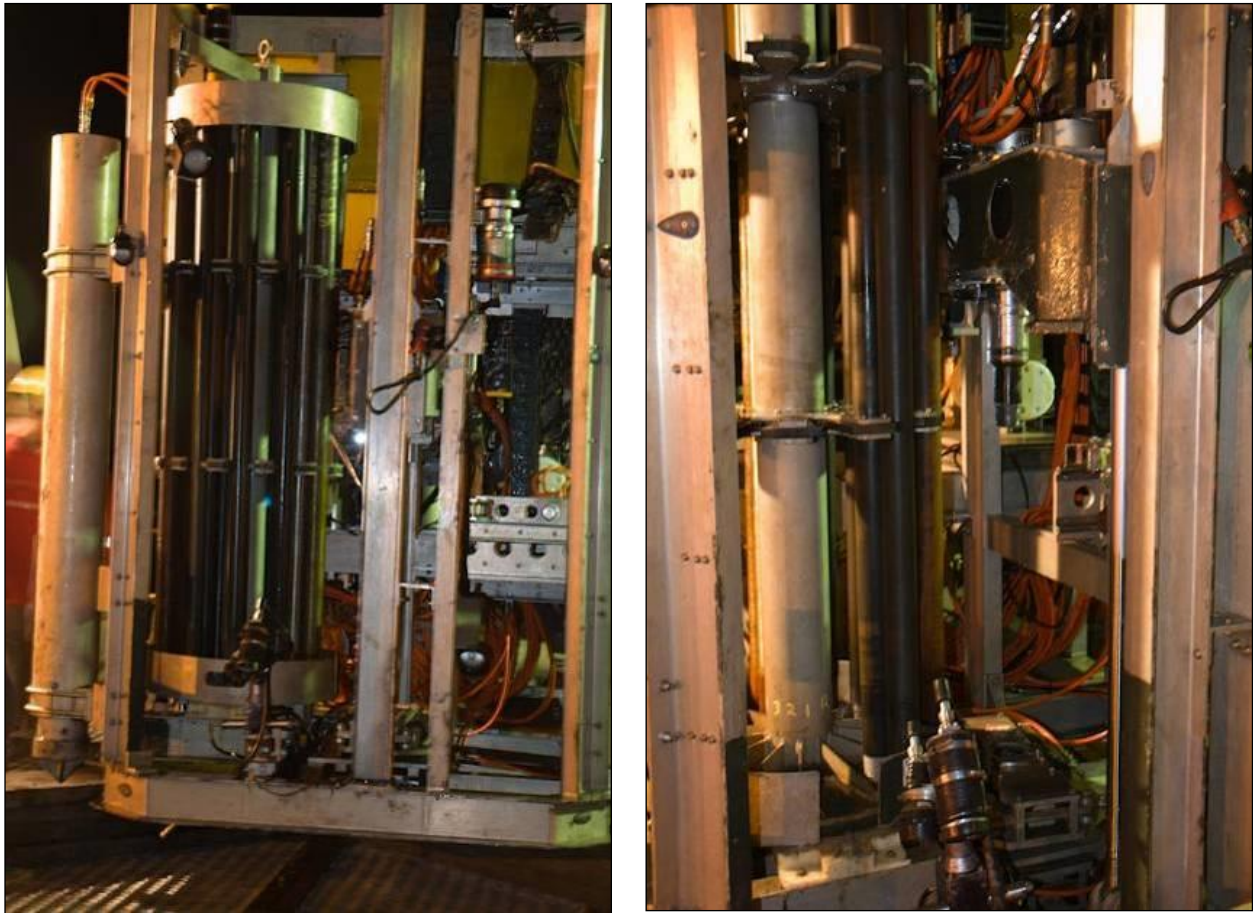
Figure 10.1 ROV Drill1 on deck showing core barrels held in the carousel.
