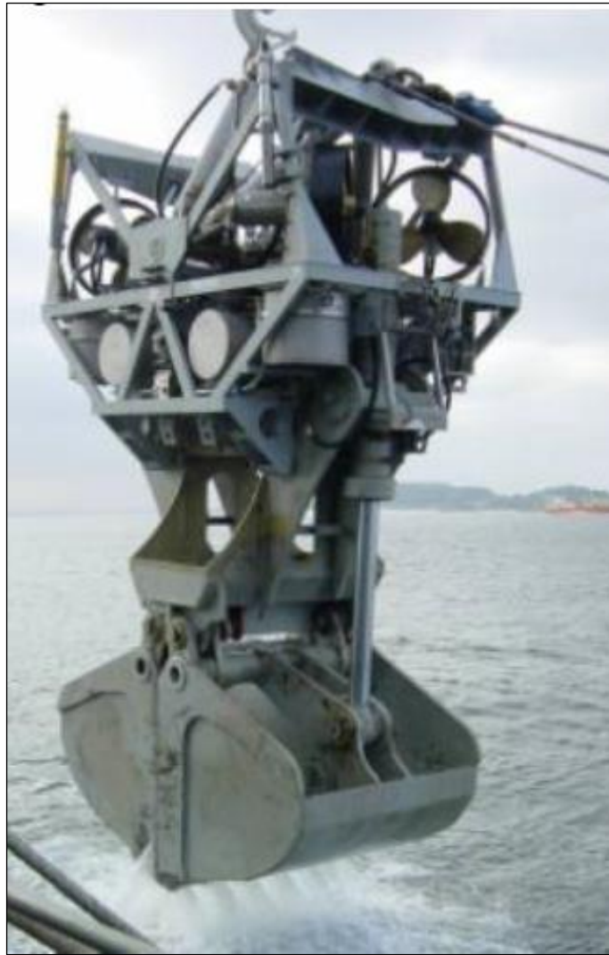
Figure 16.11 Example of clamshell excavator
