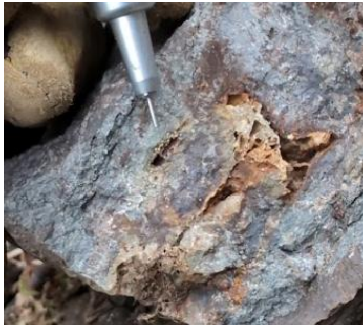
Figure 9.30 – Visible Gold in Oxidized Vug (Sample B03976 from Creek zone)
