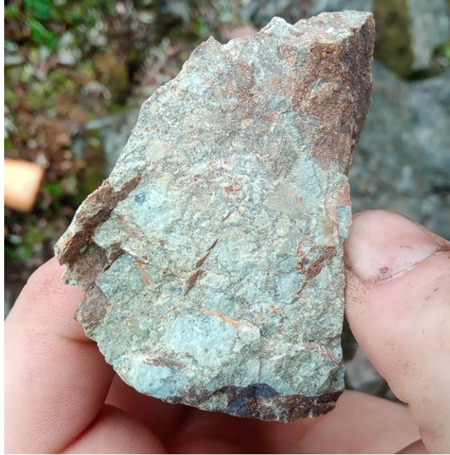
Figure 9.30 – Visible Gold in Oxidized Vug (Sample B03976 from Creek zone)
