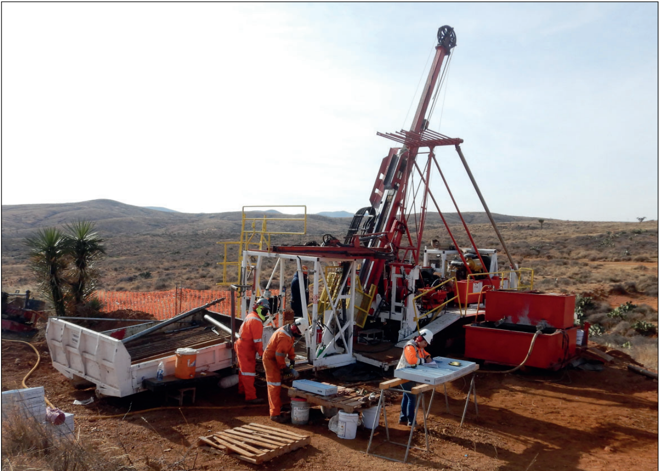
Figure 22: Major 50 VD 6000 drill rig at Panuco North. The rig is drilling HQ diameter core. Core recovery and geotechnical logging is conducted at site — before core is moved to the companies drill logging and storage facility in Zacatecas. Drilling is being conducted by Major Drilling.
