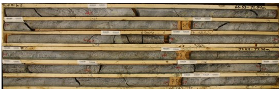
Figure 2: Rush-001 - Discontinuous intersections of semi-massive and massive sulphide from 70.15 - 73.5m
