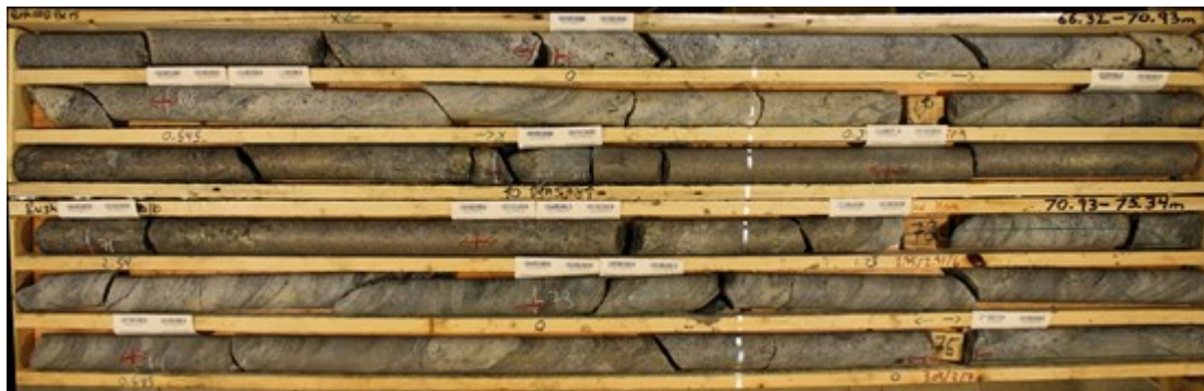
Figure 3: Rush-002 - Semi-massive and massive sulphide over 2.7m beginning at 69.25m
