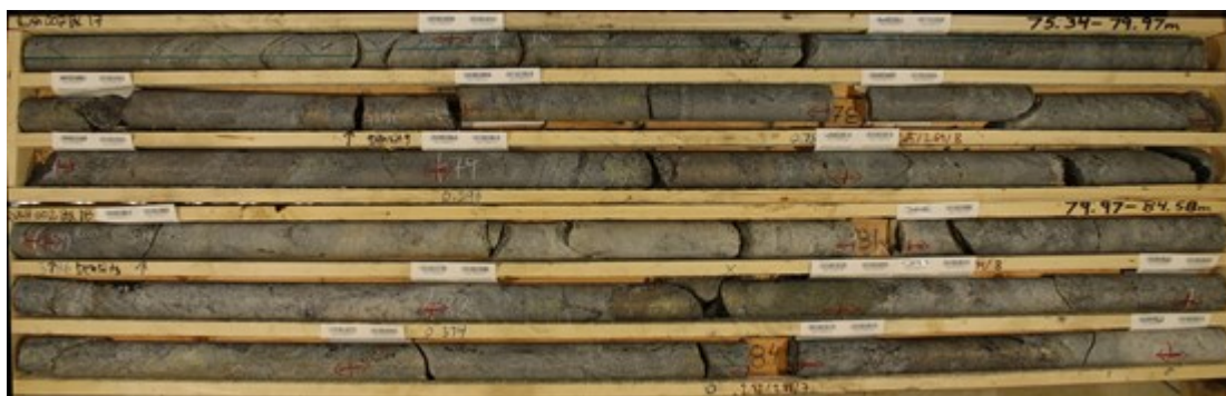
Figure 4: Rush-002 - boxes 17 and 18 showing discontinuous semi-massive to massive sulphide mineralization
