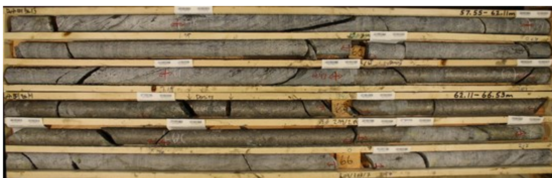
Figure 1: Rush-001 Massive Sulphide Intersection at 61.50-64.69m depth
