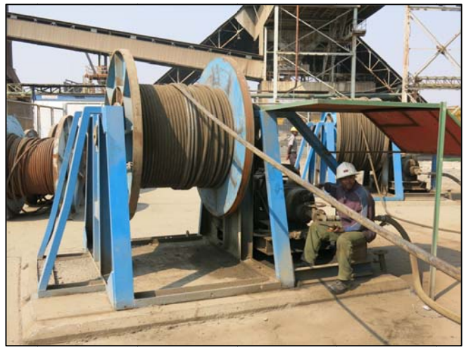
Figure 9 (left): Fabrication of platforms and ladders for emergency escapes in shafts P2, P2Bis and P15. Figure 10 (right): Shaft P5 rope take-up spool during testing of refurbished gearbox.
