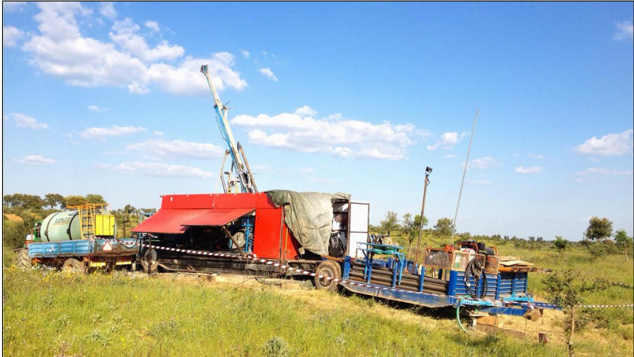
Figure 10-3: Diamond Drilling Operations at Sesmarias
