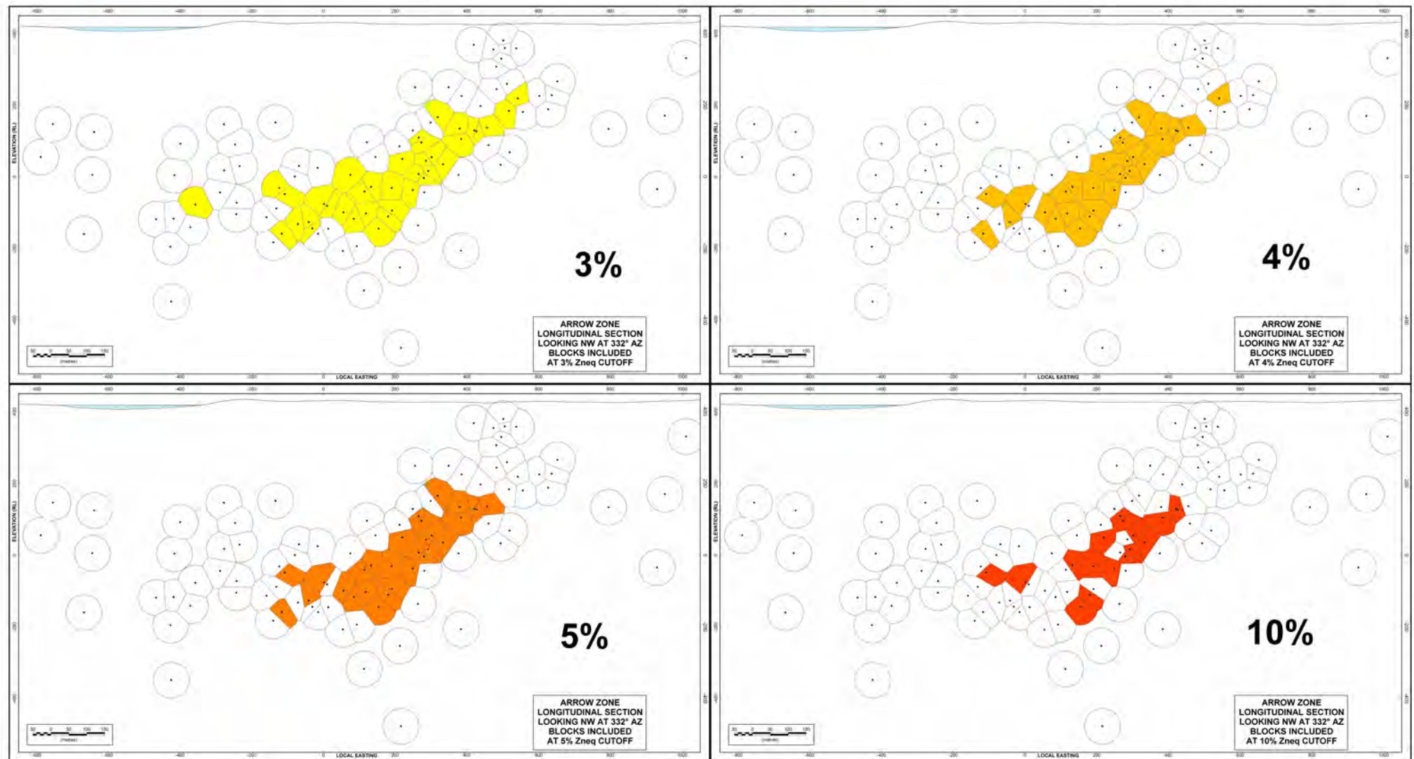
Figure 14.2: Illustration of changing cutoff grade. Blocks selected for inclusion in resource using cutoff grades of 3%, 4%, 5% and 10% Zinc equivalent
