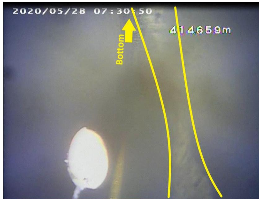
**Figure 37: Vein contact at 414.659 m (measured by the depth sensor), orientation specified with the fishing sinker**
