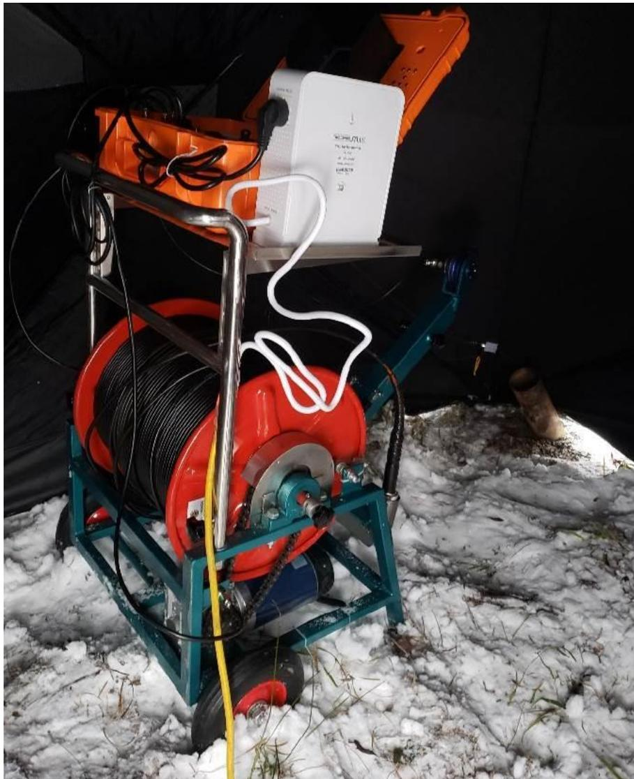
**Figure 30: 600 m borehole inspection camera, Zhengzhou Defy Robot**
