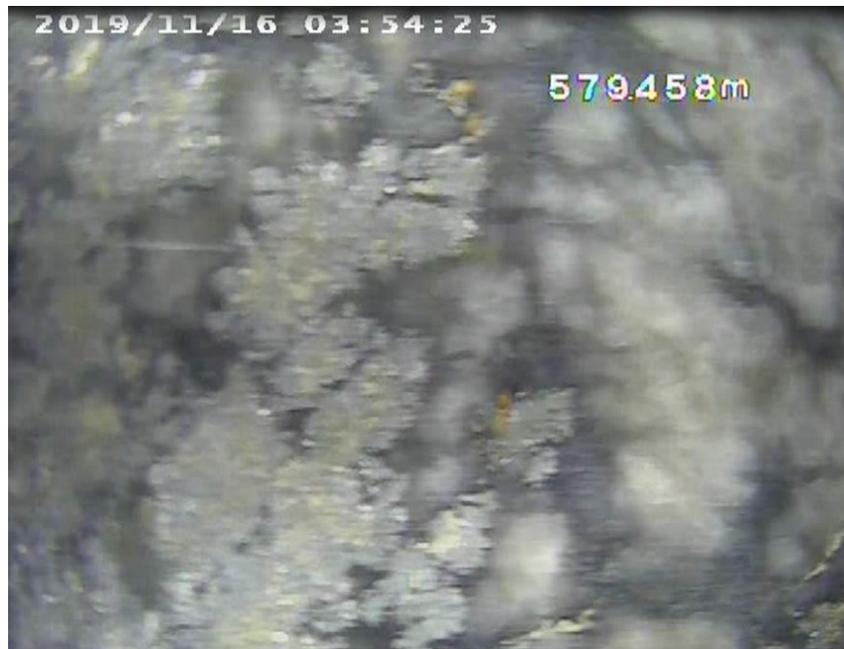
**Figure 33: Silver Mineralization in the vein lateral camera view at 579.46m**
