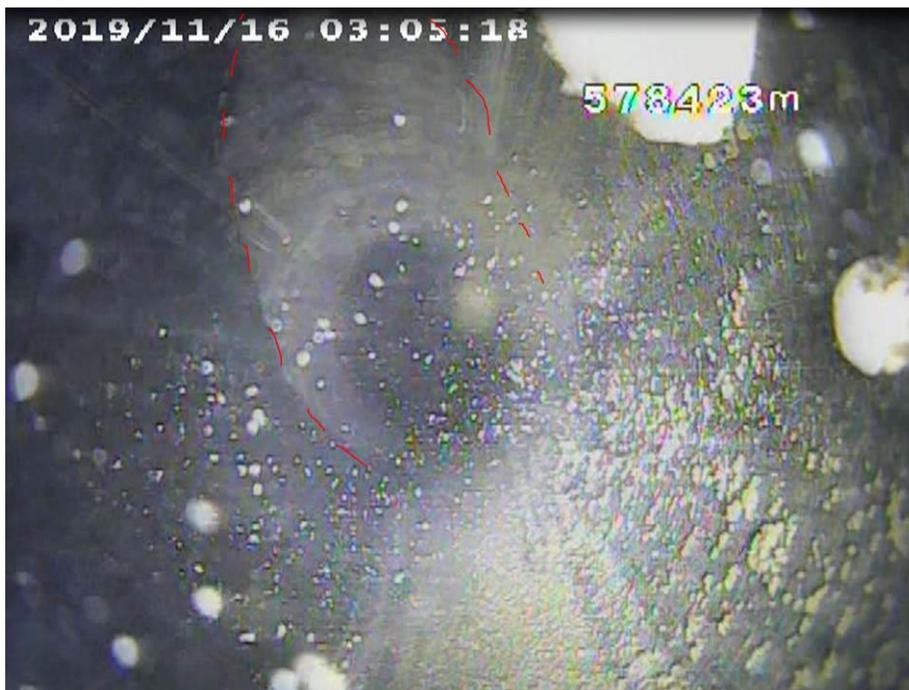
**Figure 32: Vein contact with weight at 2 O'clock and contact at 11 O'clock**
