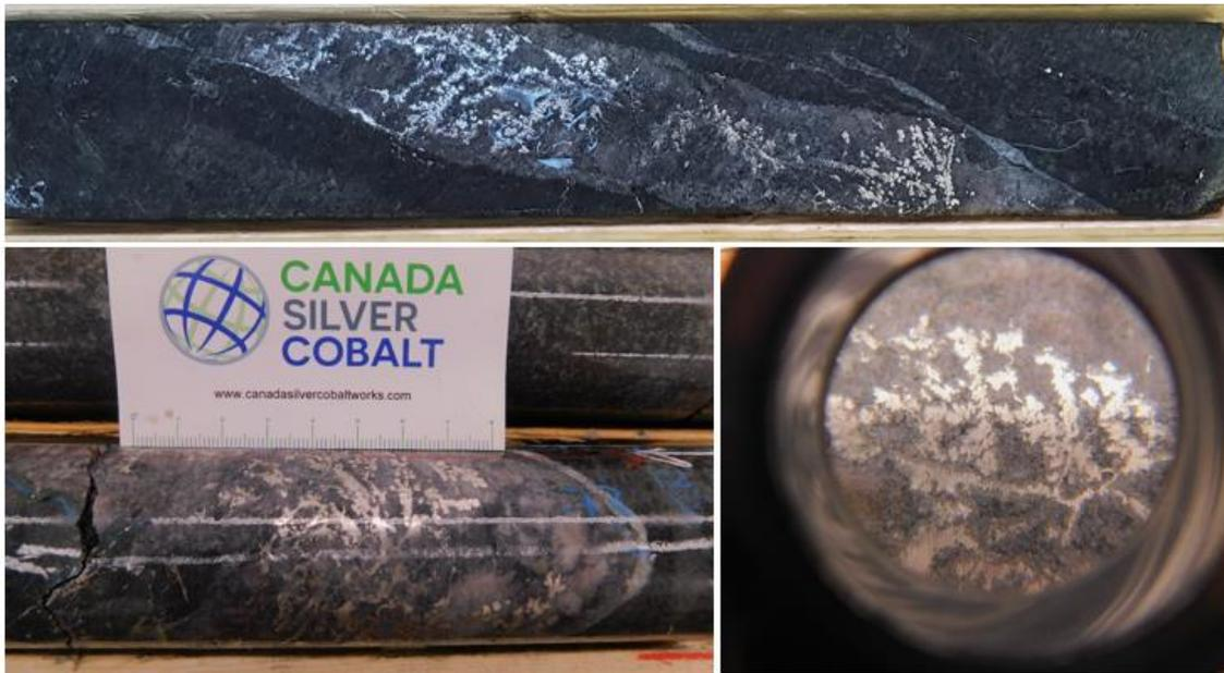
**Figure 44 : Massive vein showing silver-cobalt mineralisation in hole CS-20-39**
