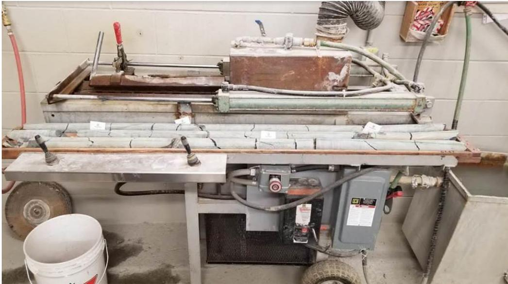
**Figure 49: Electrical saw used for cutting the core samples**
