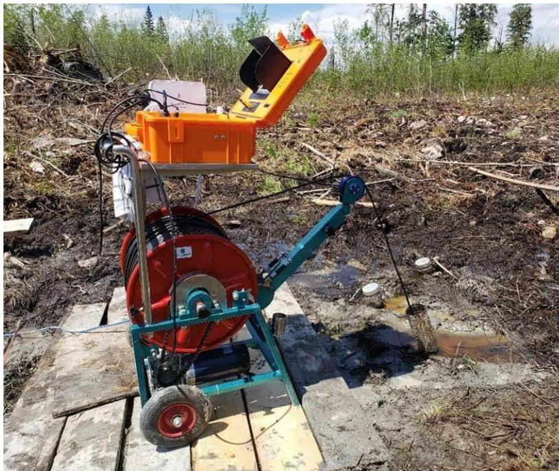
**Figure 36: The camera down hole CS-20-22.**
