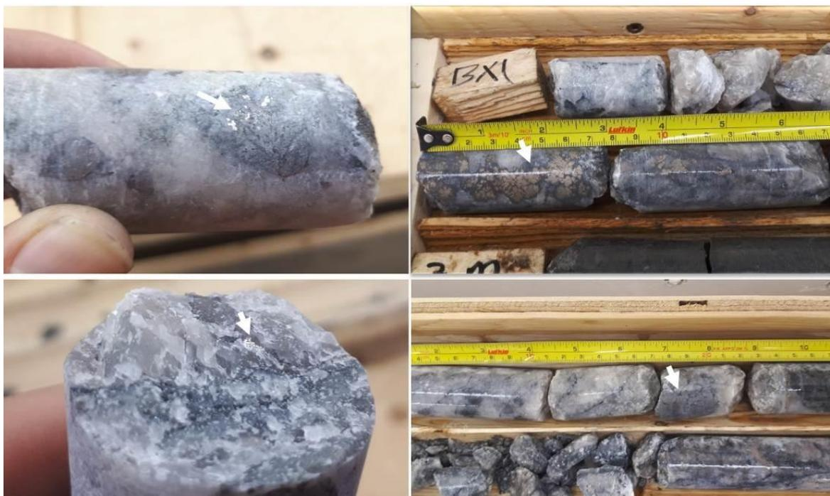
**Figure 13: Underground drill core showing silver-cobalt-nickel mineralisation (white arrows)**
