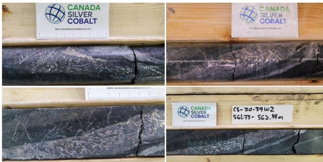
**Figure 46 : Massive vein with silver-cobalt mineralisation in hole CS-20-39W2**
