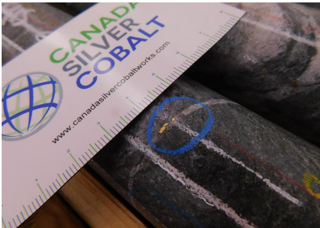
**Figure 43 : Visible gold at hole CS-20-31**
