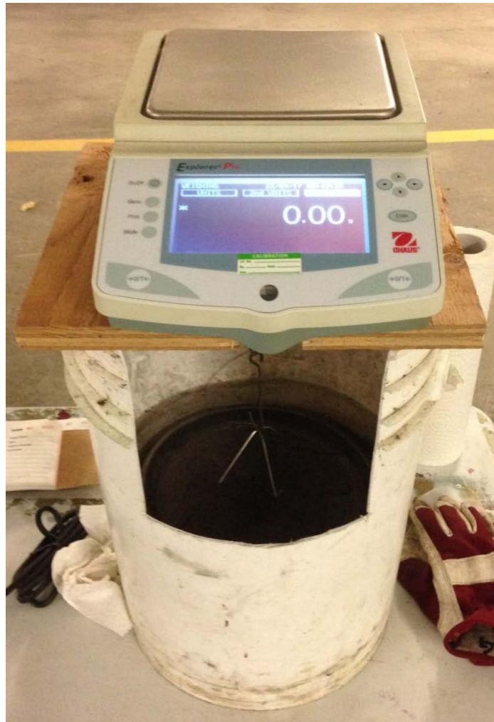
Figure 12-3 Balance scale and water bucket setup for measuring specific gravity of core (Source: Blind Creek, 2018)
