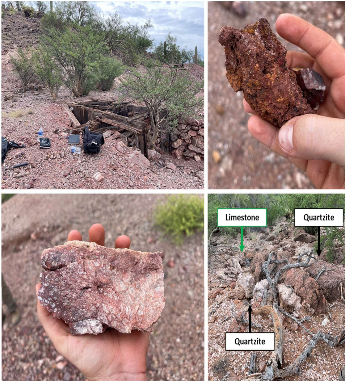
Figure 36. Top left: Picture of the old working at the El Cobre; Top right: Gossan breccia in tailings; Bottom left: quartz vein brecciated in mine dumps; Bottom right: Outcrop near the mine with similar interbedding of limestone and quartzite
