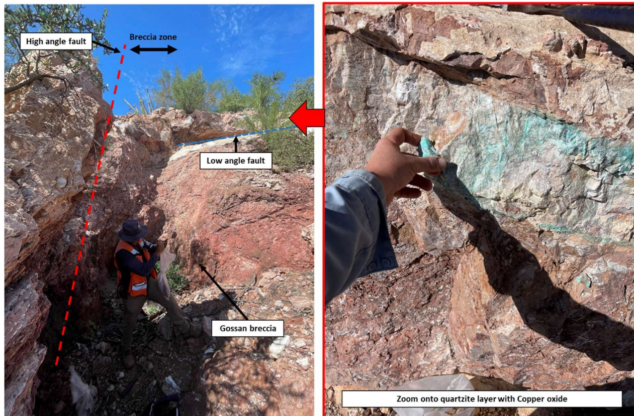
Figure 33. Photo showing the mineralization and relationship with structural and lithological controls at the La Union Mine.
