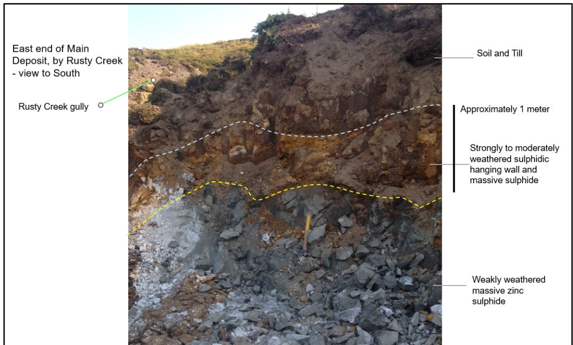
Figure 1. Eastern limit of the Main Deposit, excavation removed two meters of overburden and 1 m of weathered material to expose weakly weathered sulphides.
