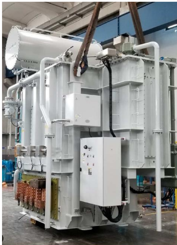
Figure 24.15 – Electrolysis Transformer FAT Test
