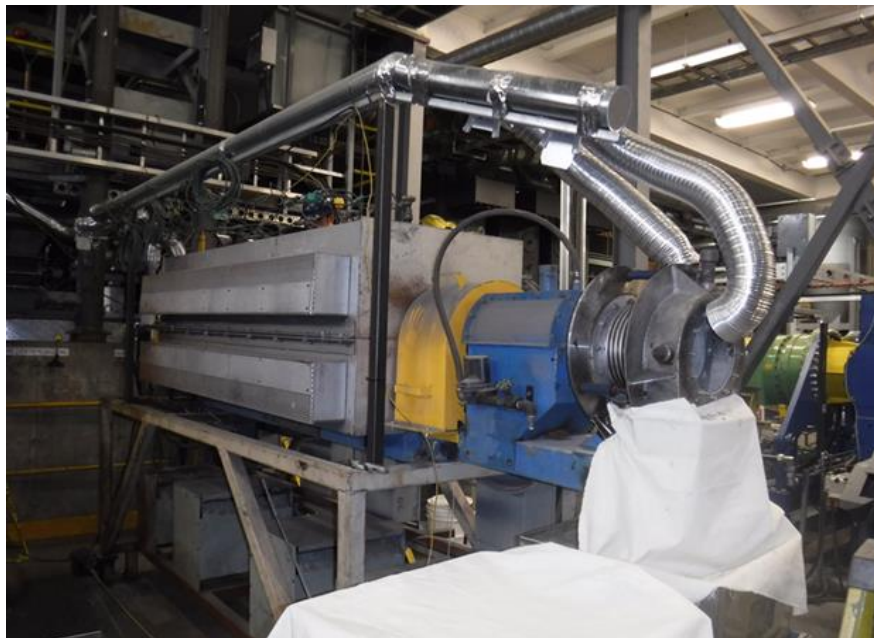
Figure 13.15 – Pilot Acid Bake Kiln at COREM
