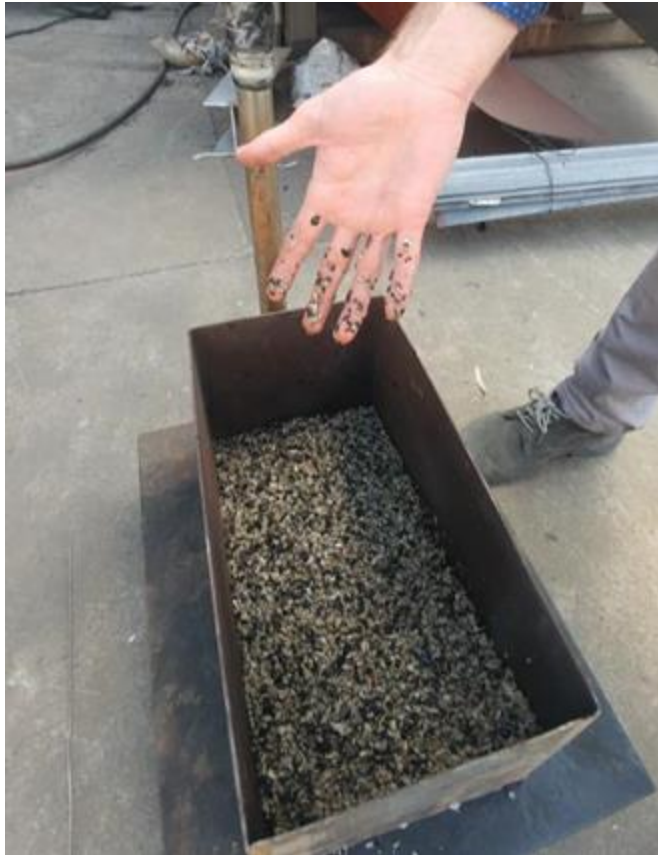
Figure 13.11 – ThermoPower Drying Test #2, 80° Discharge Temperature
