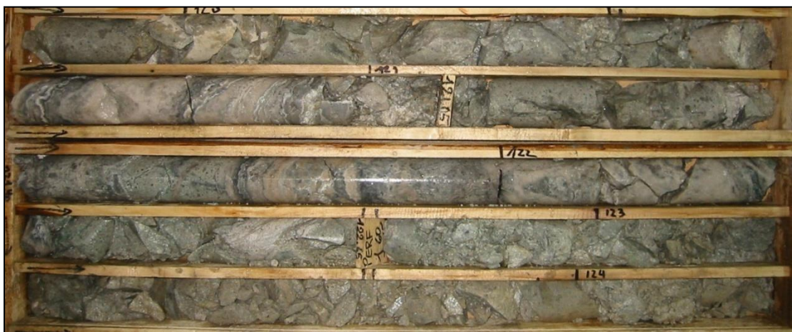
Figure 8.2 Main Quartz Vein in Hole LM-020-D (from 121.00 m and 122.50 m)
