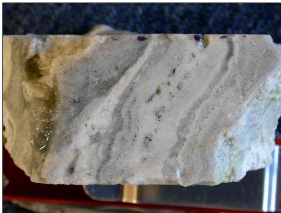
Figure 7.8 Core Sample Showing Crustified Vein Texture.
