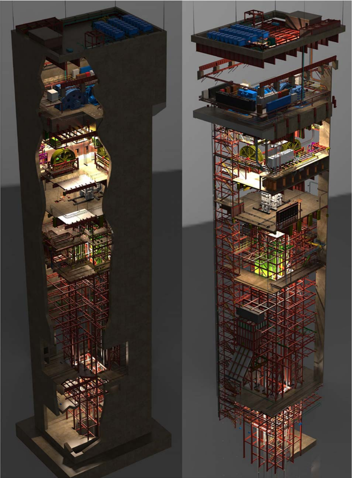
Figure 3: Illustration shows two perspectives of Shaft 2's 103-metre-tall concrete headgear, the hitch (foundation) and internal permanent hoisting facilities.
