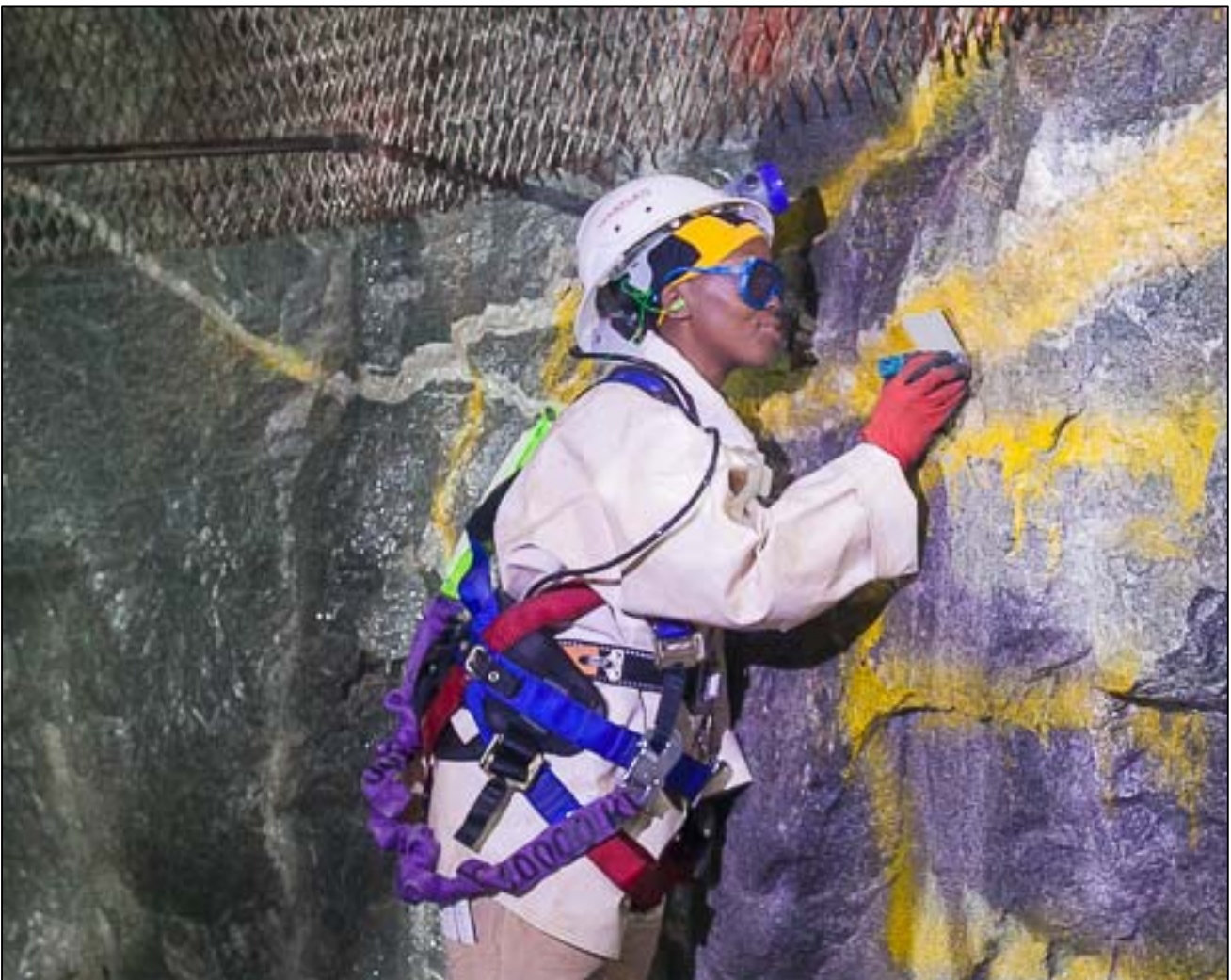
Figure 1: A Platreef engineer examining geotechnical features of the Shaft 1 sidewall.
