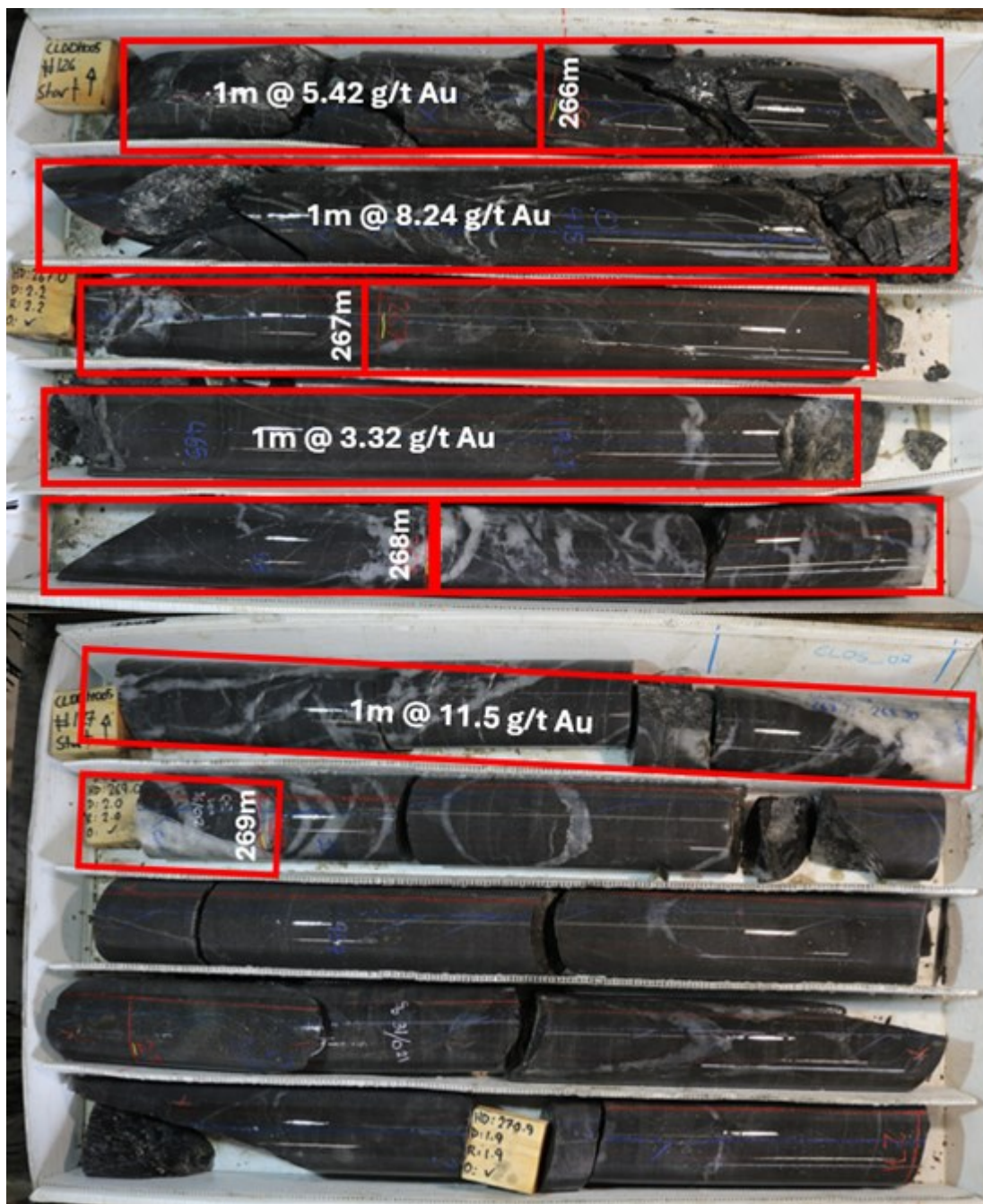
Figure 5 - Diamond drill core from CLDDH005 showing significant intervals of quartz veining and sulphide intervals
