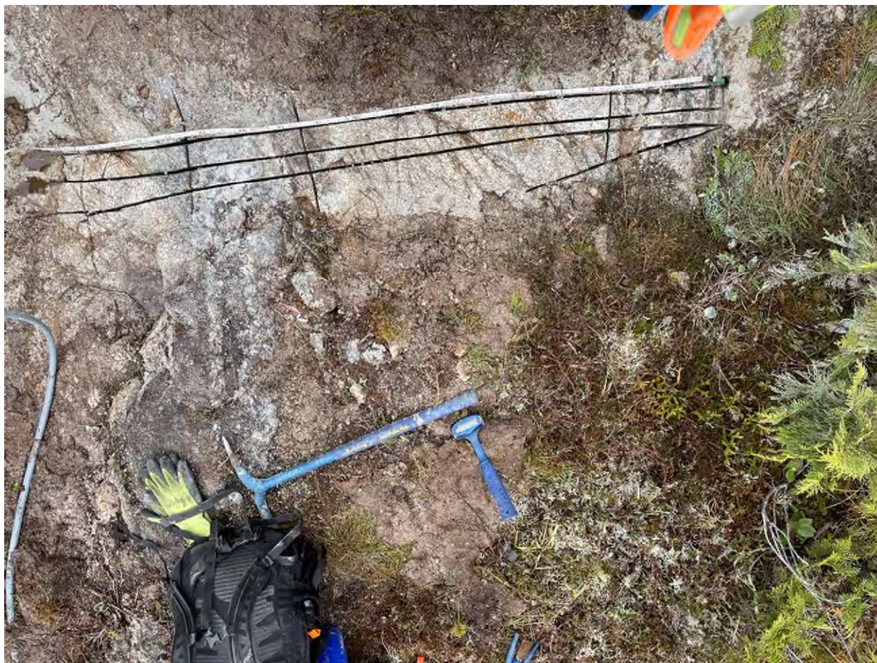
Figure 49. Typical channel sample layout after the saw cuts were made and before the samples were extracted. Handle of the pick is pointing north.
