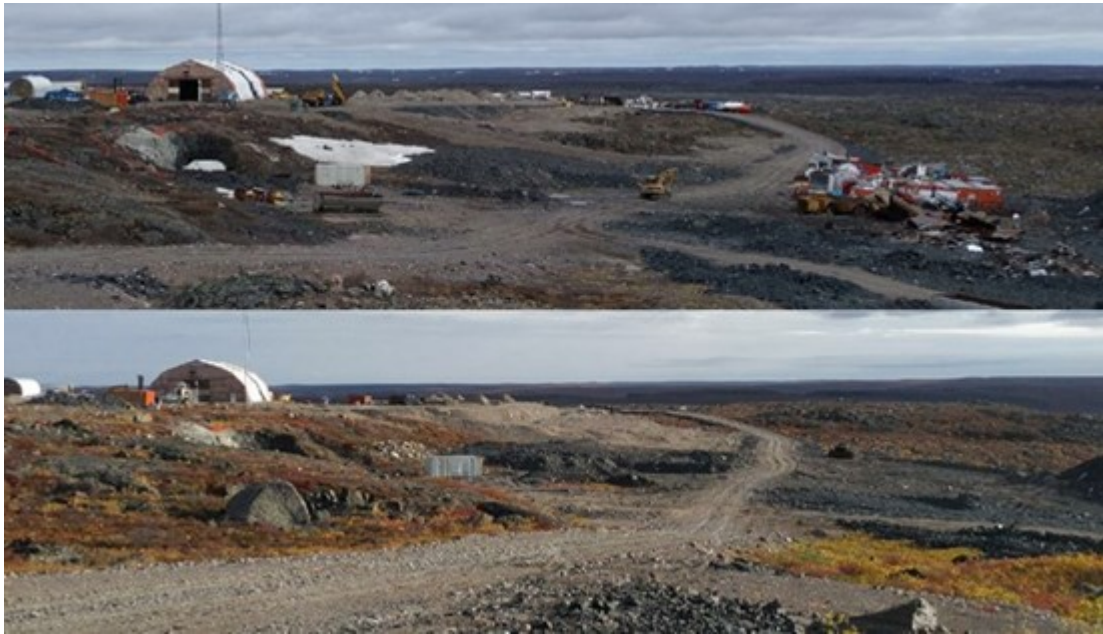
Figure 4: Change in Waste Piles from July to September 2021.
