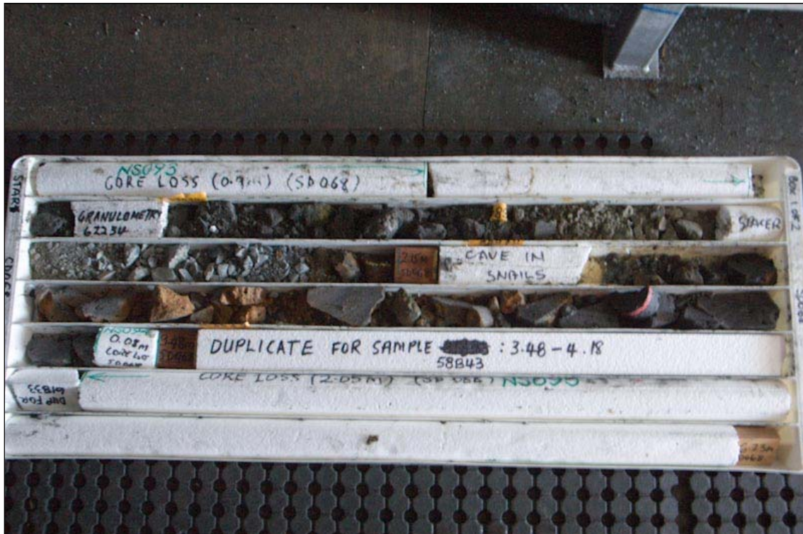
Figure 12-3: Drill storage after sampling (Hole SD068) showing half core duplicate
