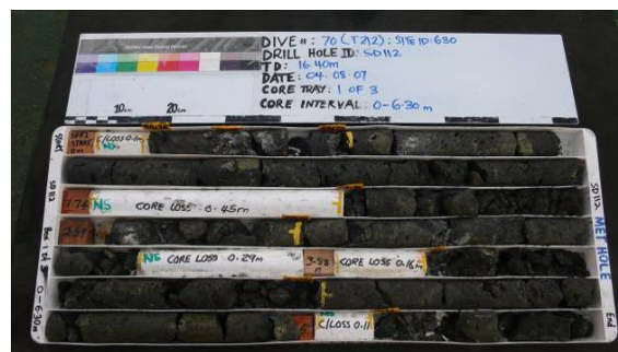
Figure 12-2: Core photos for hole SD 112 before (left) and after sample mark up (right)
