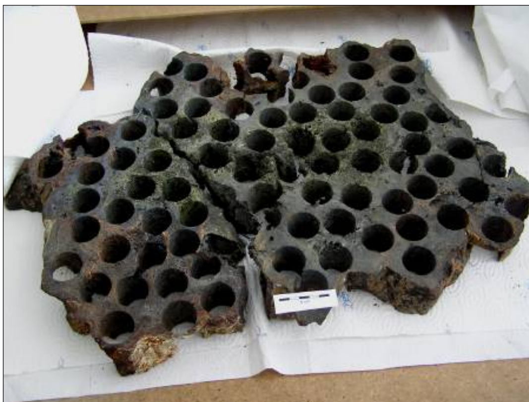
Figure 9-6: Slice through chimney with sample core holes
