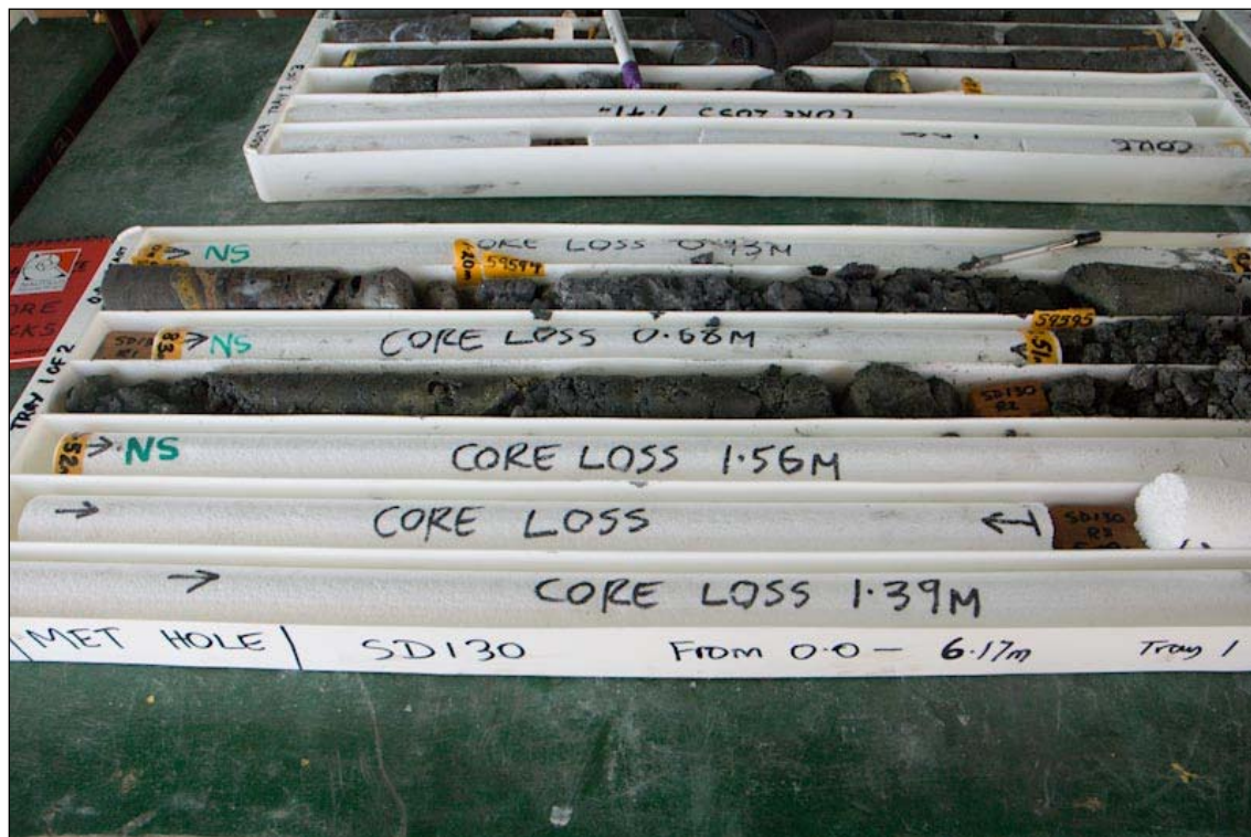
Figure 12-1: Drillcore mark up (hole SD 130) before sampling
