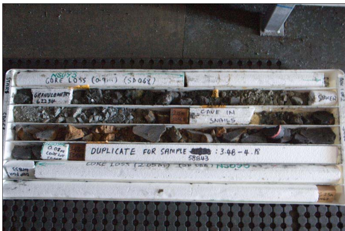
Figure 13-3: Drill storage after sampling (Hole SD068) showing half core duplicate
