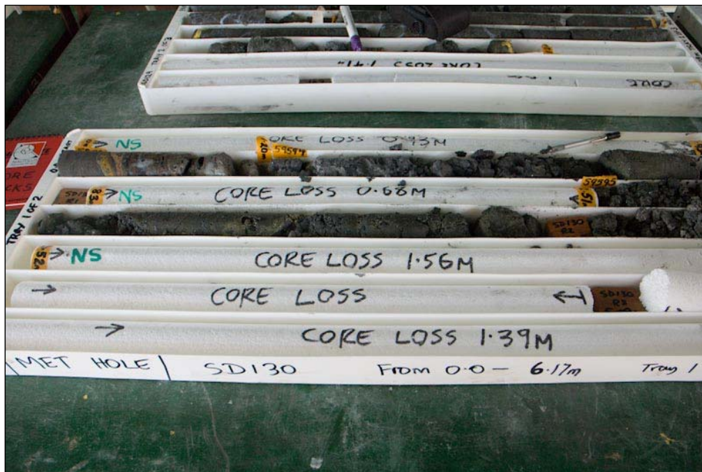
Figure 13-1: Drillcore mark up (hole SD 130) before sampling
