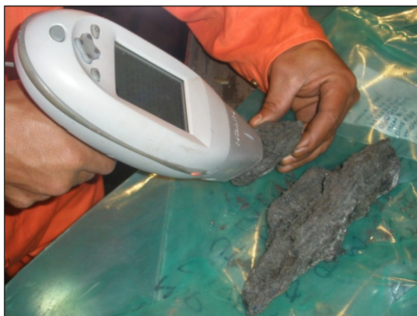
Figure 13-8: Niton handheld XRF measuring cut face of chimney sample
