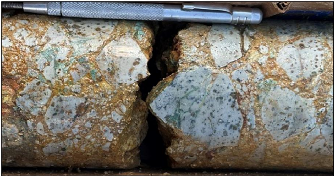
Figure 3: MHB-30 39.3 meters (129 ft)/1.5 meters (5 ft) @ 1.86% Cu and 19.4 g/t Ag
