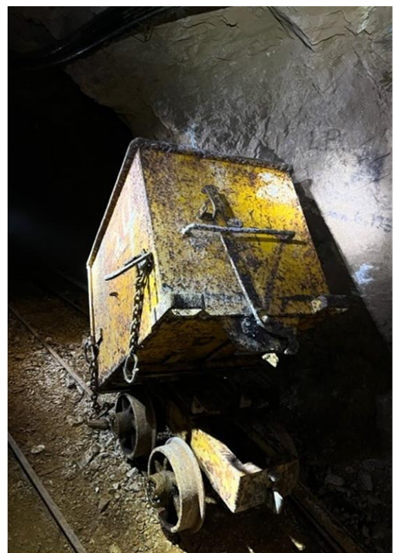
Figure 6 Shaft 1 headframe, with man cage in place (left). The shaft was used into the 1980's. An ore cart at the side of the tunnel showing tilting mechanism (right).
