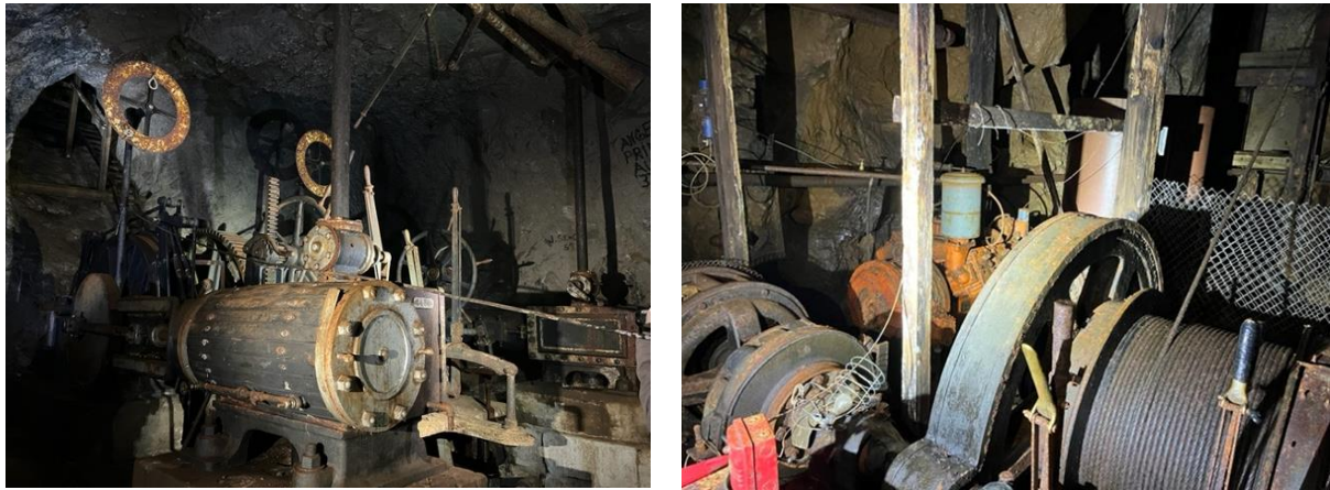
Figure 7 Original steam powered winch (left) and the 1950's replacement electric winch for Shaft 1.
