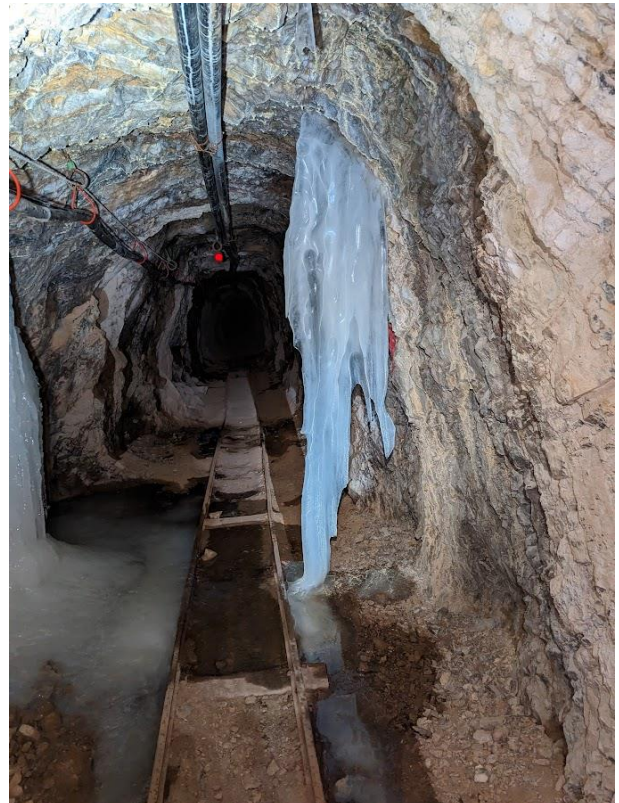
Figure 5 Supported portal area (left) and more typical unsupported underground tunnel with rails, air, power and water lines fixed to the backs (right).
