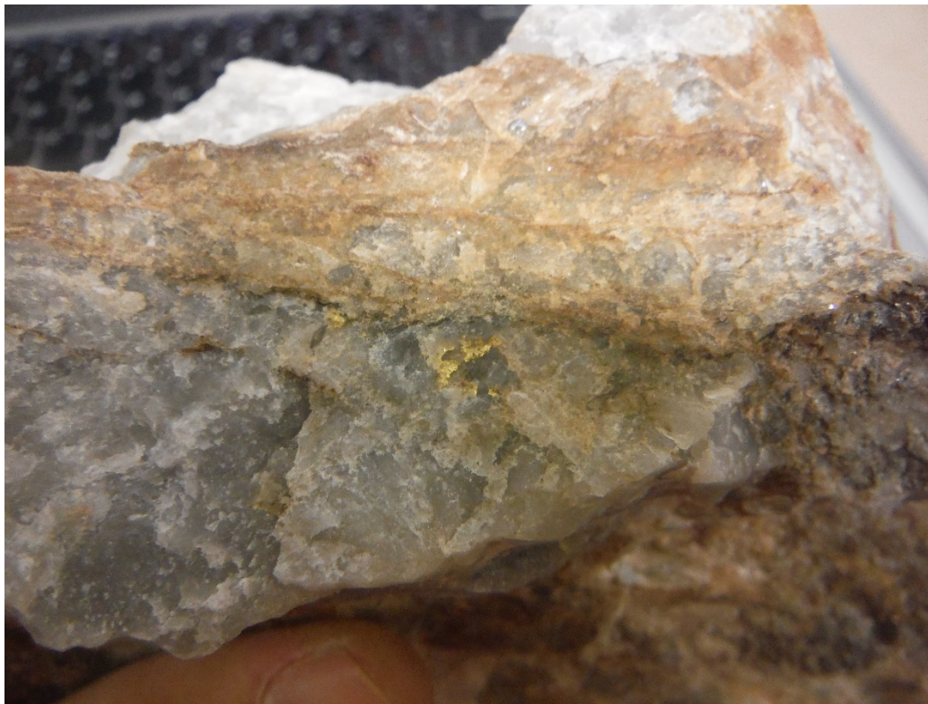
Figure 10: Visible gold within smoky quartz vein at the surface.
