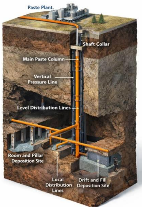
Figure 16.32: Conceptual Paste Backfill Reticulation System
