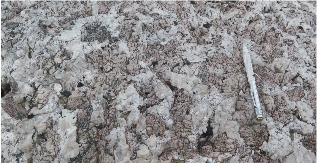
Figure 7.9: Strongly Fractured, Pinkish Weathered Spodumene Crystals in Matrix of White Feldspar and Grey Quartz at the CV5 Pegmatite
