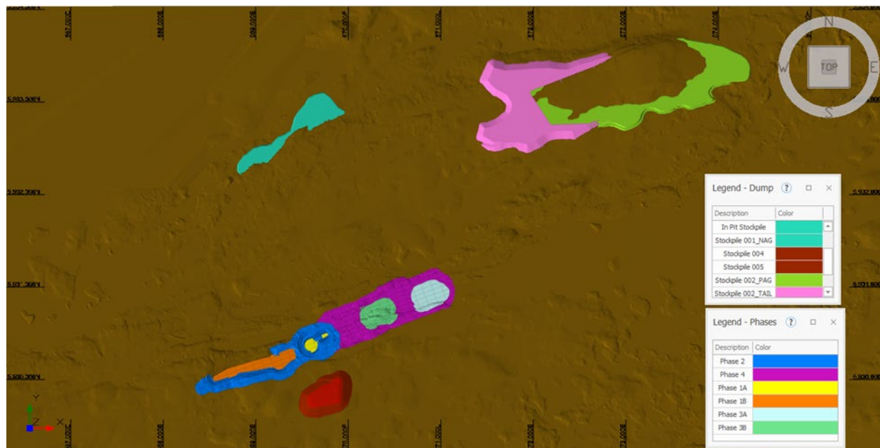
Figure 16.19: Mine Development End of June 2030– Plan View
