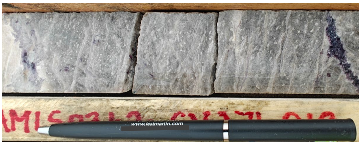
Figure 7.21: Pollucite Mineralization in High-Grade Caesium Drill Intersection at ~64.5 m Depth in Drill Hole CV23-271 at the Rigel Zone, CV13 Pegmatite
