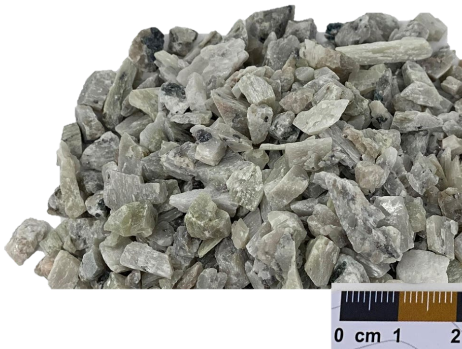
Figure 13.11: Close-up of Spodumene Concentrate (DMS + non-magnetic fractions) 5.8% \text{Li}_2\text{O} and 0.60% \text{Fe}_2\text{O}_3 at 79% Recovery
