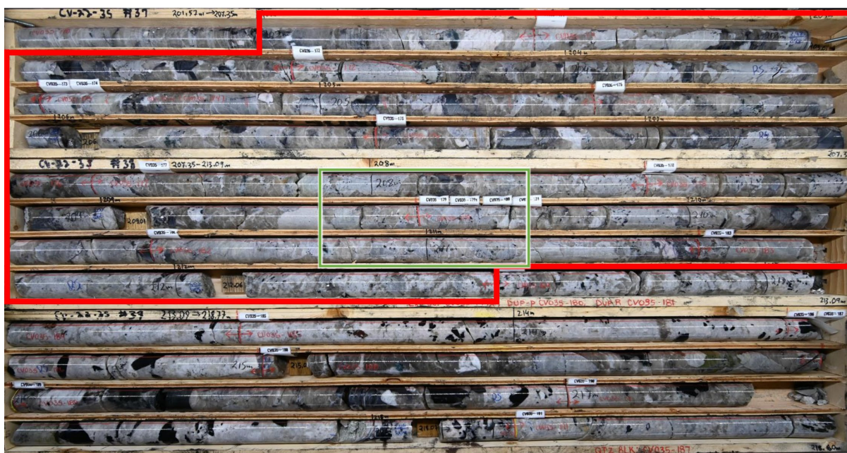
High-grade lithium mineralized drill intersection in CV22-035 – 3.29% \text{Li}_2\text{O} and 177 ppm \text{Ta}_2\text{O}_5 over 10.0 m (202.5 m to 212.5 m – red box) within a wider zone of 1.25% \text{Li}_2\text{O} and 118 ppm \text{Ta}_2\text{O}_5 over 96.9 m (126.1 m to 223.0 m)
