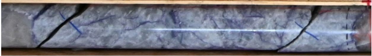
Figure 7.22: Pollucite with Lepidolite Veining (purple) in Grey Quartz Matrix from 139.3 m to 139.5 m in Drill Hole CV24-520 (Vega Zone), Within a Wider Zone of Caesium Mineralization Grading 7.39% \text{Cs}_2\text{O} over 7.1 m
