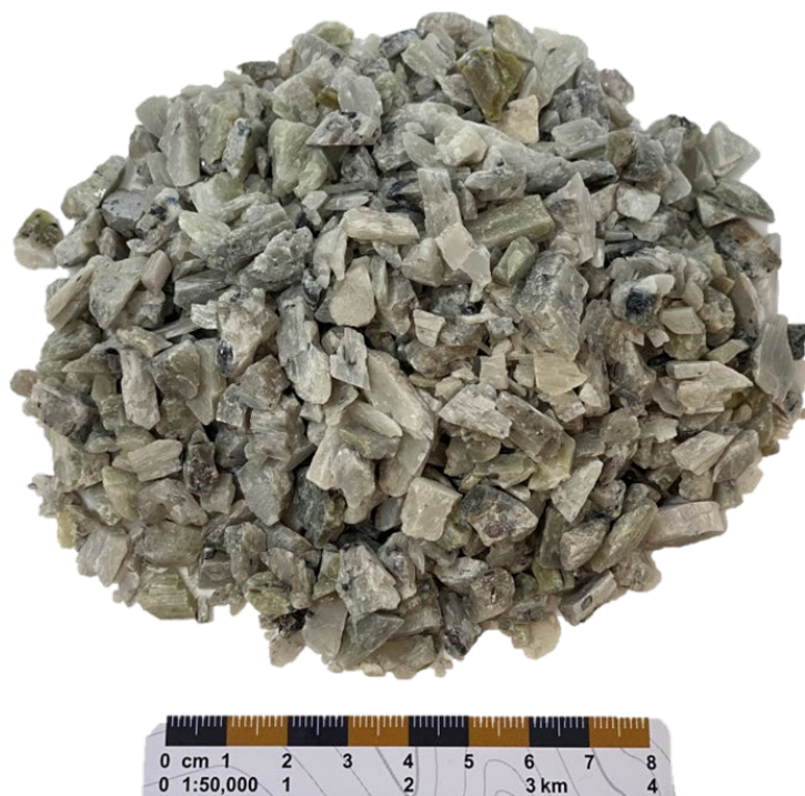
Figure 13.10: Spodumene Concentrate (DMS + non-magnetic fractions) 5.8% \text{Li}_2\text{O} and 0.60% \text{Fe}_2\text{O}_3 at 79% Recovery
