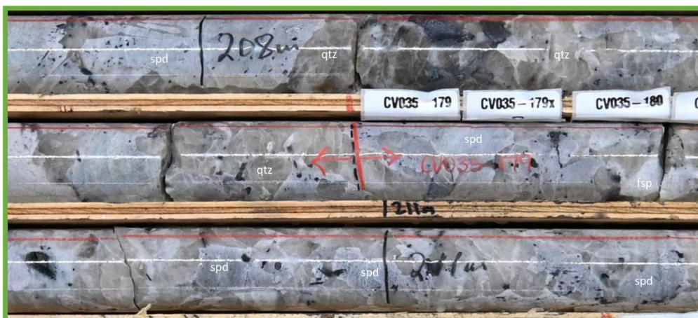
Blow-up of green box below illustrating coarse grained spodumene crystals
