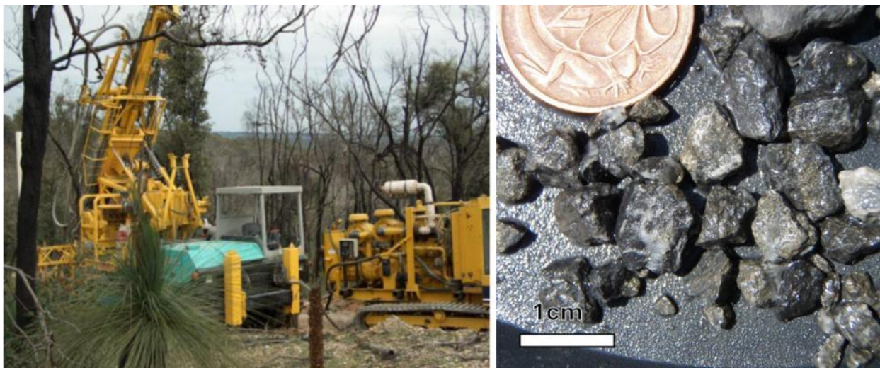
Figure 10-2 Left: Reverse-Circulation drillrig onsite at Steiglitz Project in 2008; Right: Chips showing visible sulphide mineralisation (McConachy 2009).
