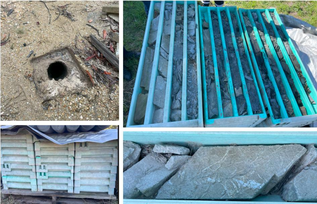
Figure 12-1 Hole STG04. Location was confirmed in the field, and the core is accessible. Core is in good condition except for some soft strongly foliated mudstones that have deteriorated.
