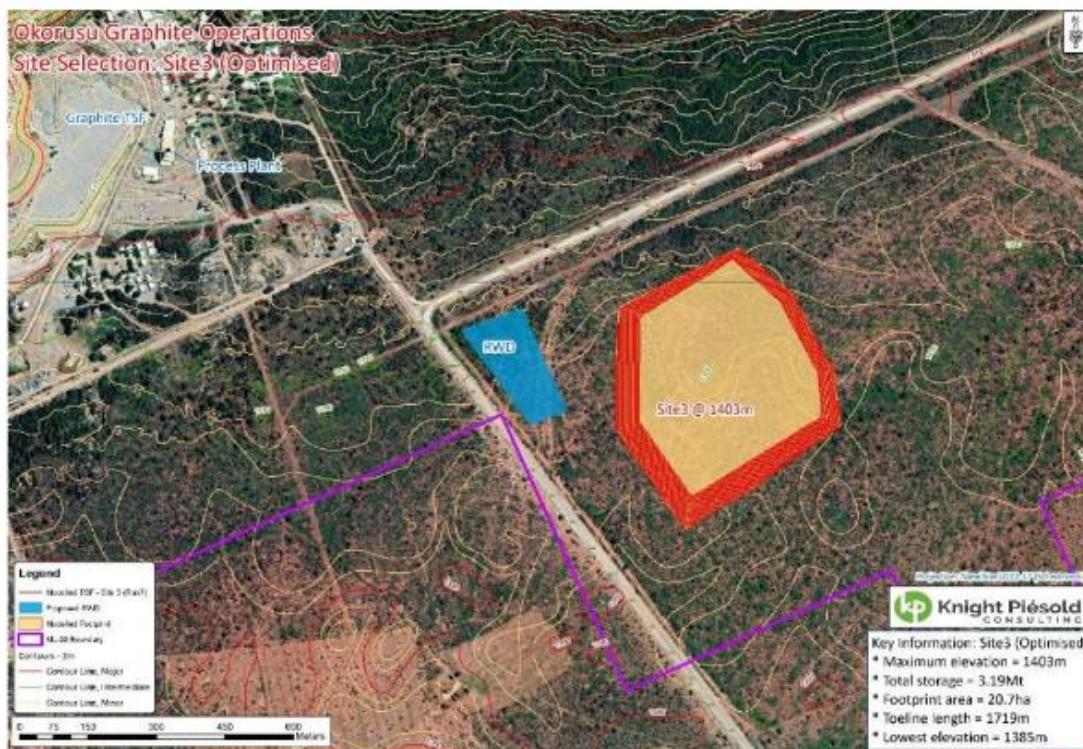
Figure 17-4: Okorusu TSF Site 3A (TSF Site 3B not indicated)
