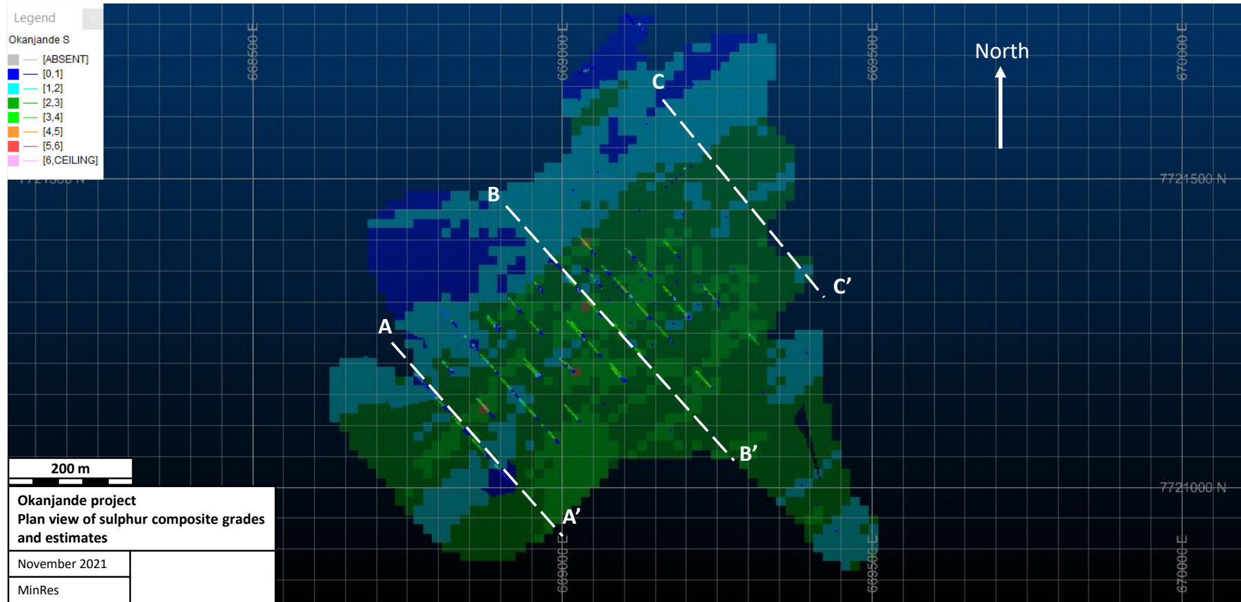
Figure 14-16: Plan view showing block model grades and composite drillhole sample grades for S (MSA, 2021)
