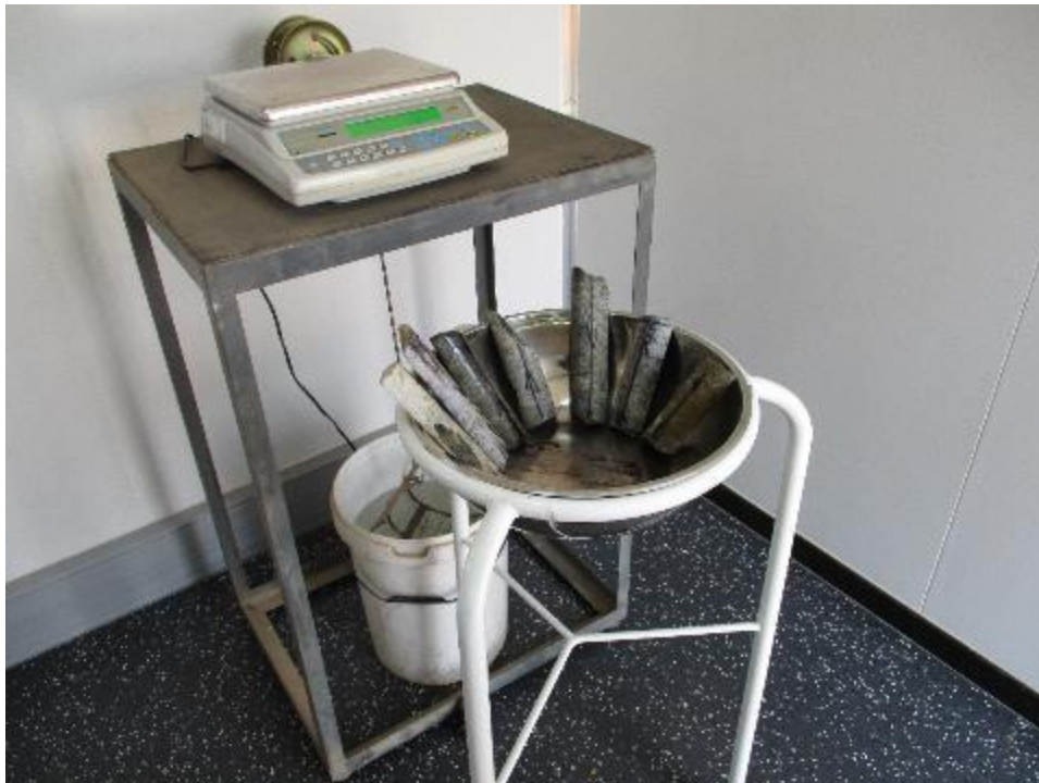
Figure 10-5: Density measurement scale and apparatus with lacquer coated core (MSA, 2021)
