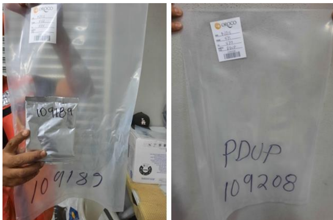
Figure 11-6: Standard Envelope with Oroco Sample Number Added and Bagged (left) and empty PDUP (pulp duplicate marker) bag (right).
