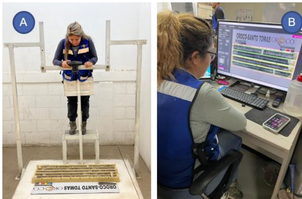
Figure 11-2: A: Core Photo Capture Station at El Ranchito; B: Core Photo Preparation and QA in IMAGO®.
