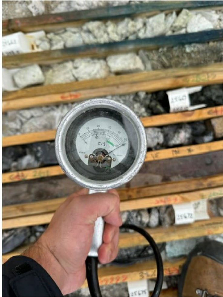
Figure 9-2: Confirmation of Mineralization via a SPP2 Scintillometer (UMR, 2024)
