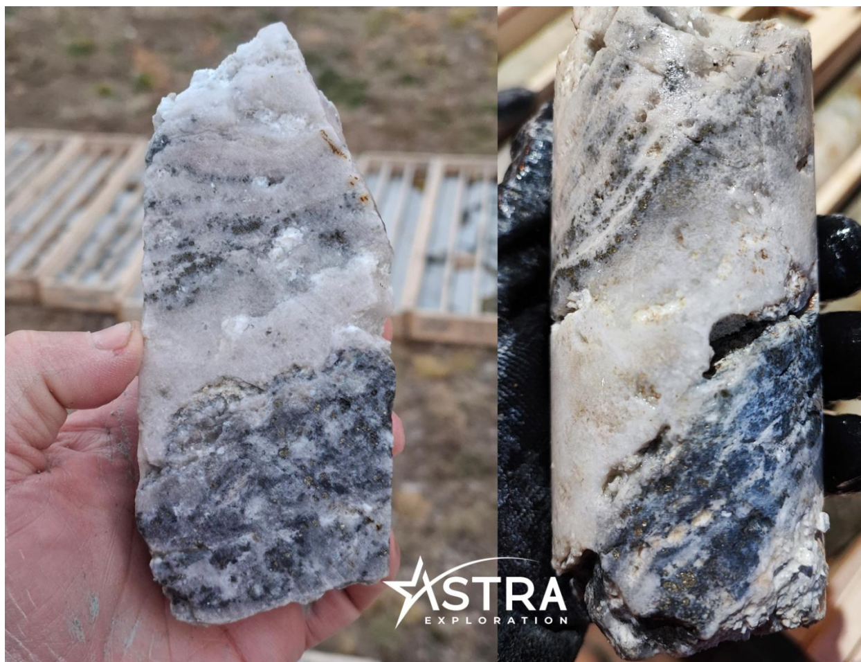
Photo 1: Banded quartz and black sulphides vein from hole LMD-107A grading 199.3 g/t Au + 228 g/t Ag approximately 150m below surface.
