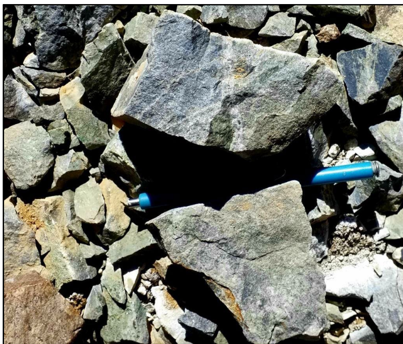
Figure 12.3 E436884 N6844469. Andesite with moderate pervasive magnetite-sericite-chlorite alteration with quartz veinlets and Cu-oxides
