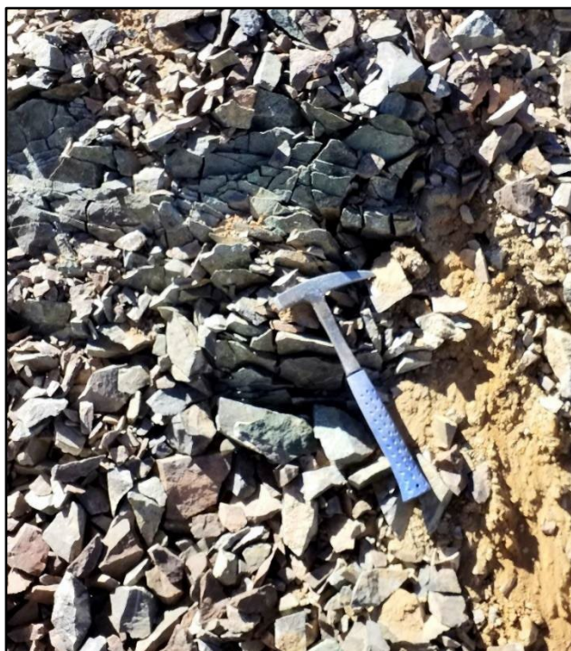
Figure 12.16 E439884 N6844469. Andesite with moderate-per magnetite and sericite, chlorite, chalcopyrite veinlets and traces of quartz veinlets. Cu oxide. Outcrop chip
