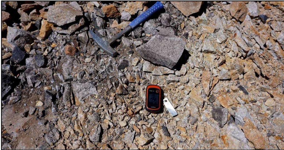
Figure 12.11 E436468 N68942100. Dacite porphyry with moderate quartz sericite, weak Potassic, Cu oxide disseminated and on Fractures 0.5%, Mag 2%
