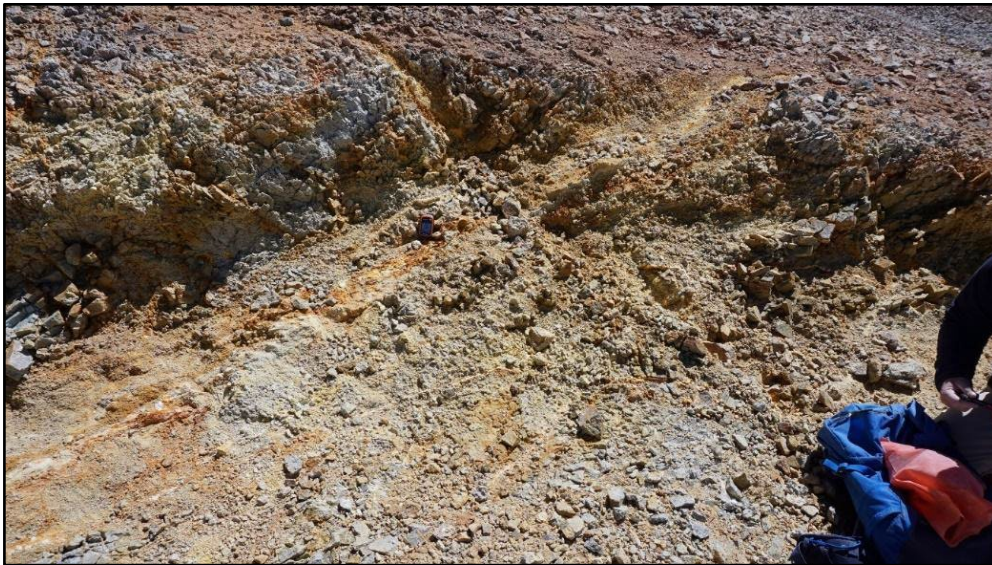
Figure 12.12 E436572 N6841951. Dacite porphyry, pervasive quartz sericite, weak Potassic in phenocrysts. Fe oxide. Fault/Structure Dip Azimuth 000o 1.5m wide. Outcrop Chip
