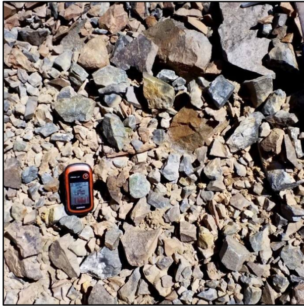
Figure 12.13 E437012 N6844682. Andesite with Cu oxide. Fine Grained. disseminated magnetite and chalcopyrite. Weak to Moderate Potassic. Float
