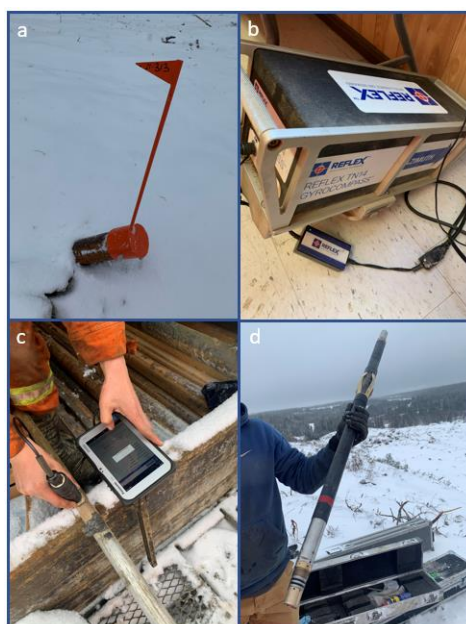
Figure 12-2. a) Drill hole marked in the field; b) Gyrocompass tool used to orient the drill rig; c) Driller demonstrating the downhole trajectory measurement procedure; d) DGI technician demonstrating OTV procedure.
