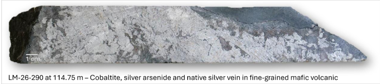
Figure 7. Core box photographs of hole LM-26-290 from 111.0 m to the end of hole (EOH) at 123.35 m, including silver assay results.
