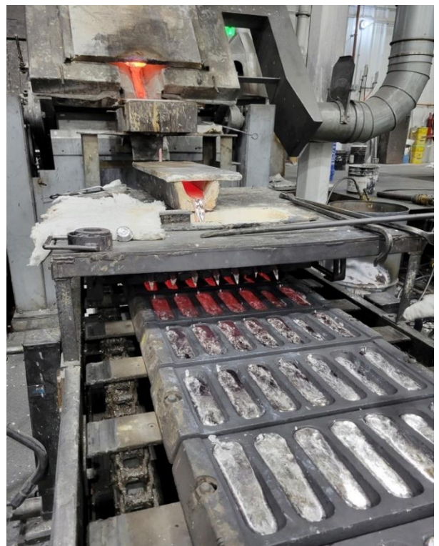
Ingots of 0.2% Aluminum-Scandium alloy being cast at IBC's foundry in Franklin, Ind.
