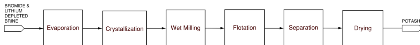
Figure 13.3: Potash Recovery Process Block Flow Diagram
