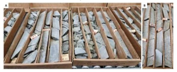
A) and B) Iron Creek typical well preserved drill core, with excellent recovery in waxed cardboard drill core box with : hole identification, box number, from-to meterage (footage) on the core box, drill-run and recovery separator drillers blocks (wood, plastic or metal) in the box, and EOH marker blocks;
