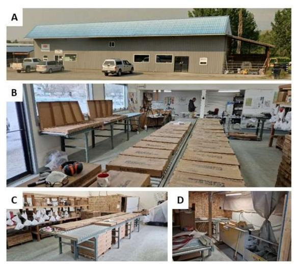
A) Issuers' core shed on I-28 in Salmon, ID (photo Google Earth); B) Efficient ergonomic core logging benches properly set-up for safe and comfortable core logging, C) temporary storage racks and D) confined core cutting and sampling lab.
