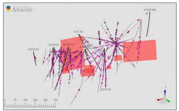
from Electra; red planes are modeled from EM data; dipping towards viewer; looking southeast Figure 9-4 – 3D View of Modeled EM-Response Plates
