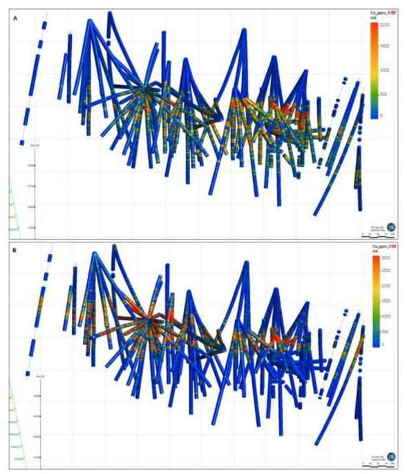
Figure 7-10 – Distribution of A) Co and B) Cu grades in the Iron Creek deposit
