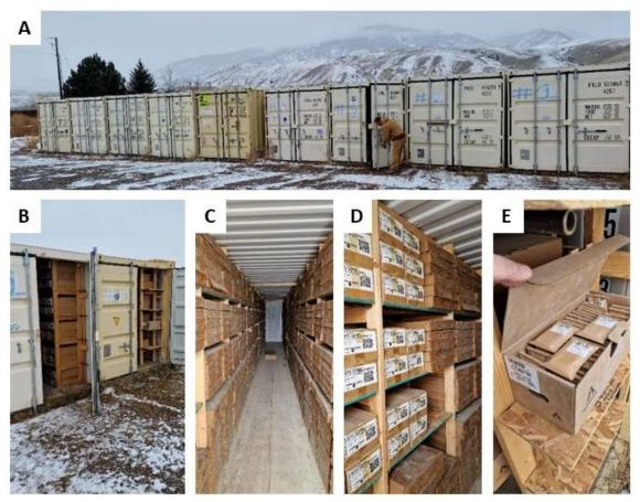
A and B) Secured core and pulp storage sea-containers in Salomon, Idaho; C) Dill core stored in organised core boxes in sea-containers; D) Stored pulp samples and drill core stored in the locked sea-container; E) Secured, well organized and documented pulps returned from ALS Laboratories to the Issuer in Salmon, ID;
