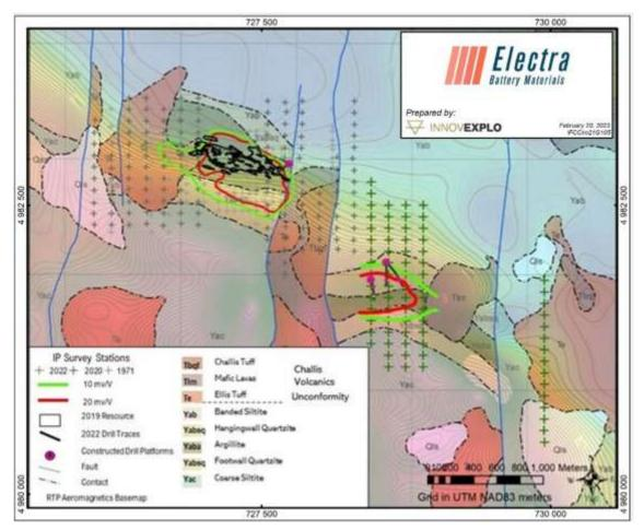
Figure 9-2 – IP Survey stations on Iron Creek and Ruby
