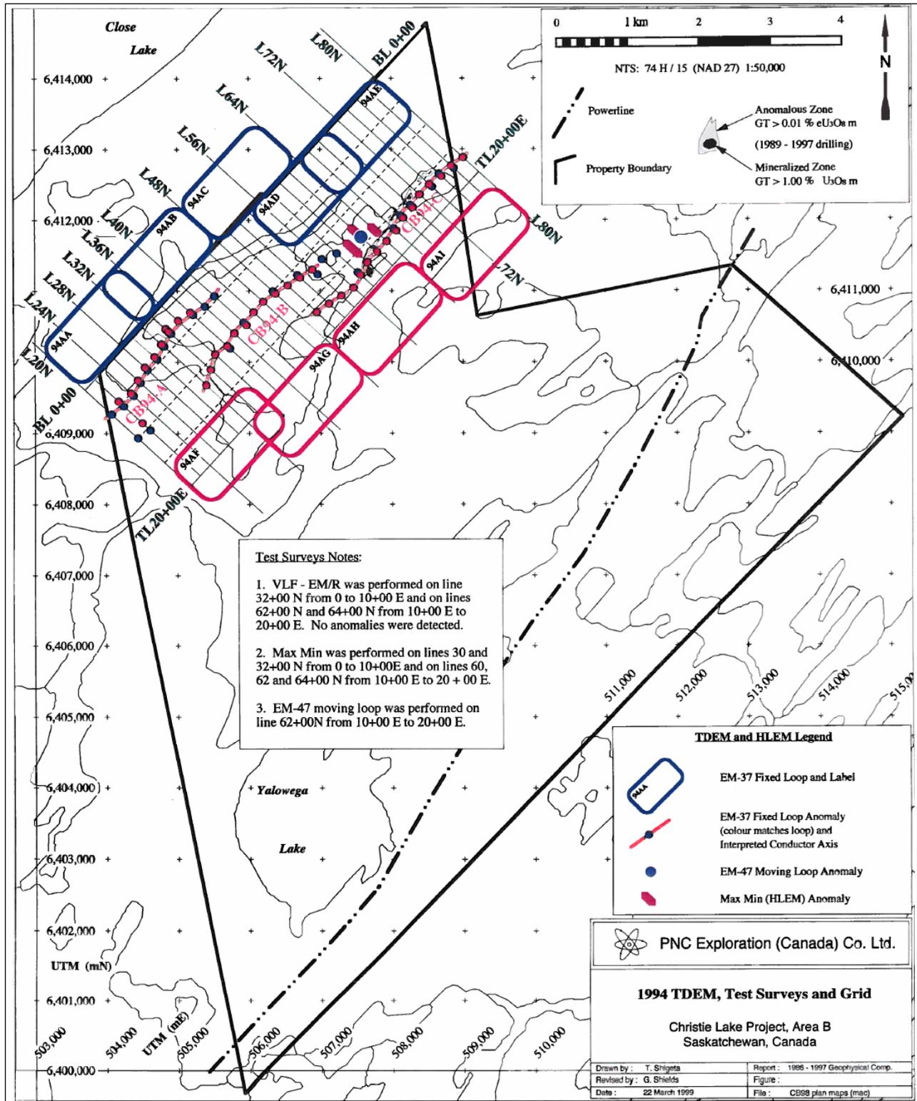
Figure 5: TDEM Surveys and Grid on the Christie Lake Uranium Project by PNC (1994)
