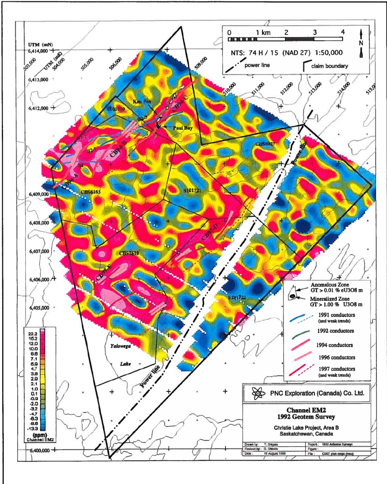
Figure 8: Channel EM2, GEOTEM Survey on the Christie Lake Uranium Project by PNC (1982)
