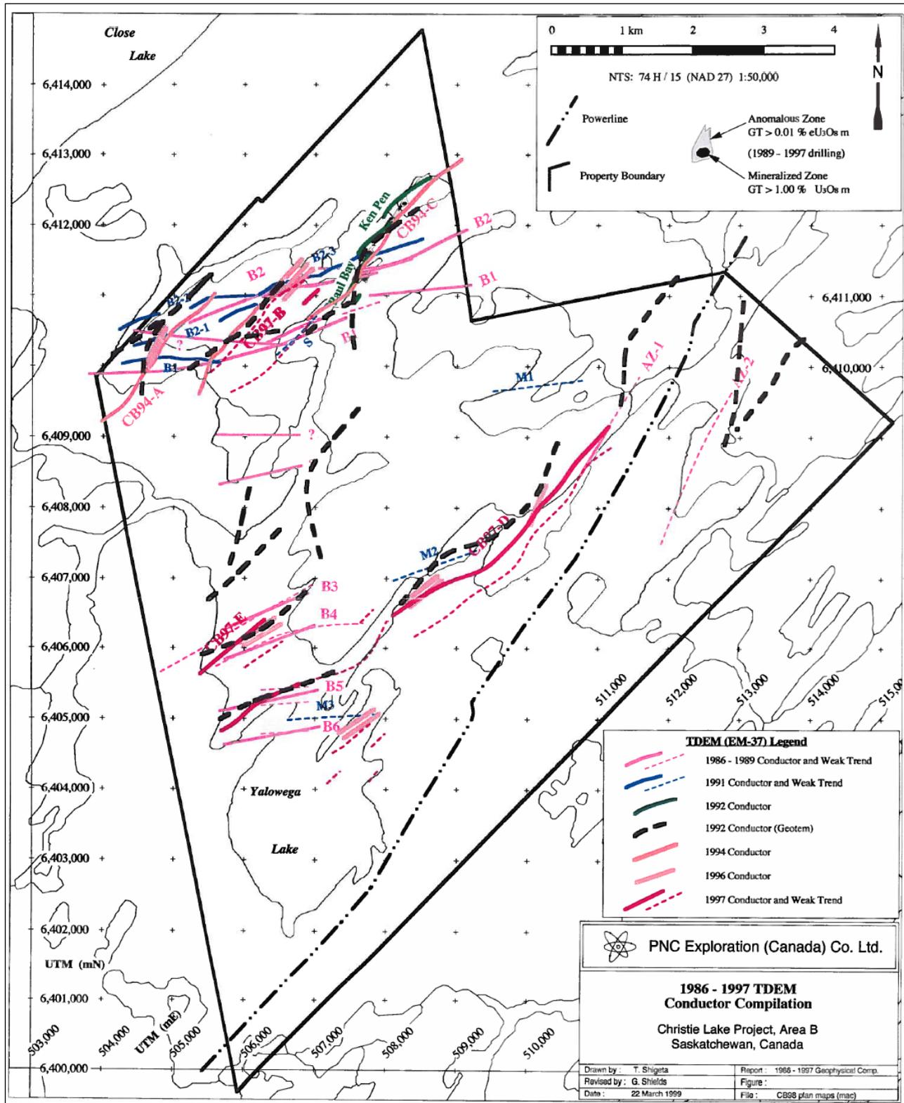
**Figure 7: Compilation of 1986-1997 TDEM Conductors on the Christie Lake Uranium Project Conducted by PNC**
