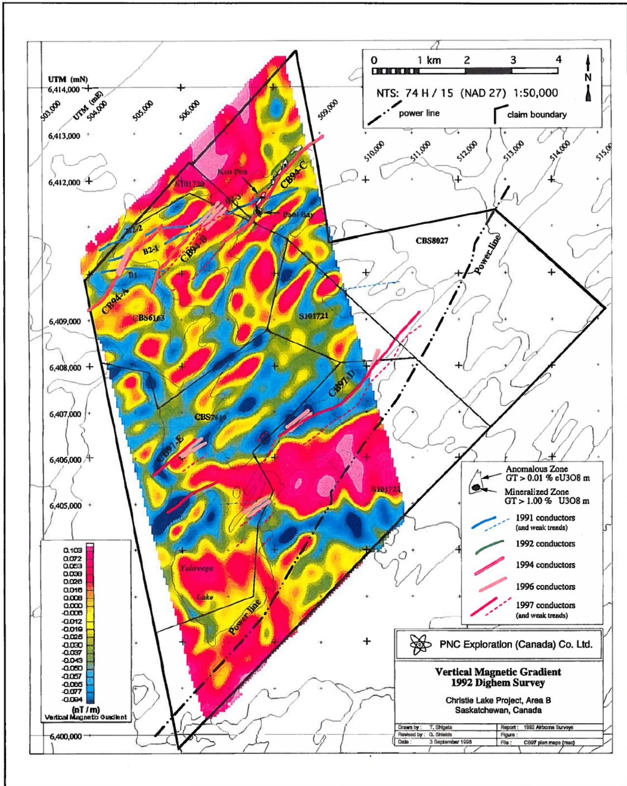
**Figure 9: Vertical Magnetic Gradient, DIGHEM Survey on the Christie Lake Uranium Project by PNC (1992)**
