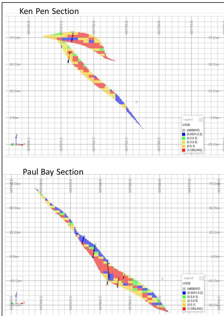
**Figure 34: Illustrative Resource Model Sections Across the Ken Pen (Top) and Paul Bay (Bottom) Mineral Resource Domains, Showing U<sub>3</sub>O<sub>8</sub> Grade Continuity Above Reporting Cut-off Grade (0.2 % U<sub>3</sub>O<sub>8</sub>)**
