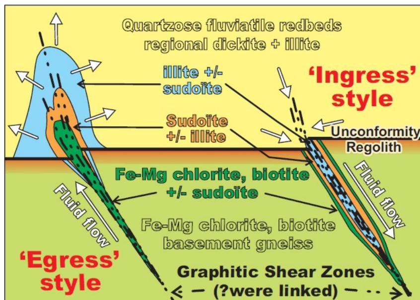
Figure 15: Unconformity Related Deposit Models
