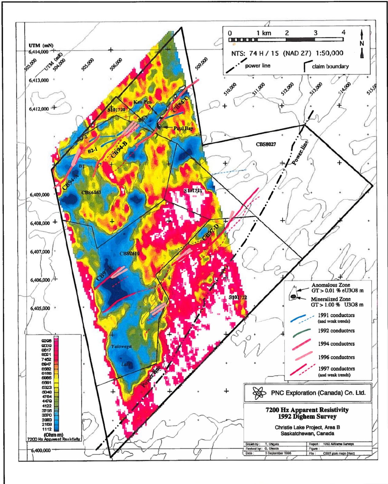
**Figure 10: 7200 Hertz Apparent Resistivity, DIGHEM Survey on the Christie Lake Uranium Project by PNC (1992)**
