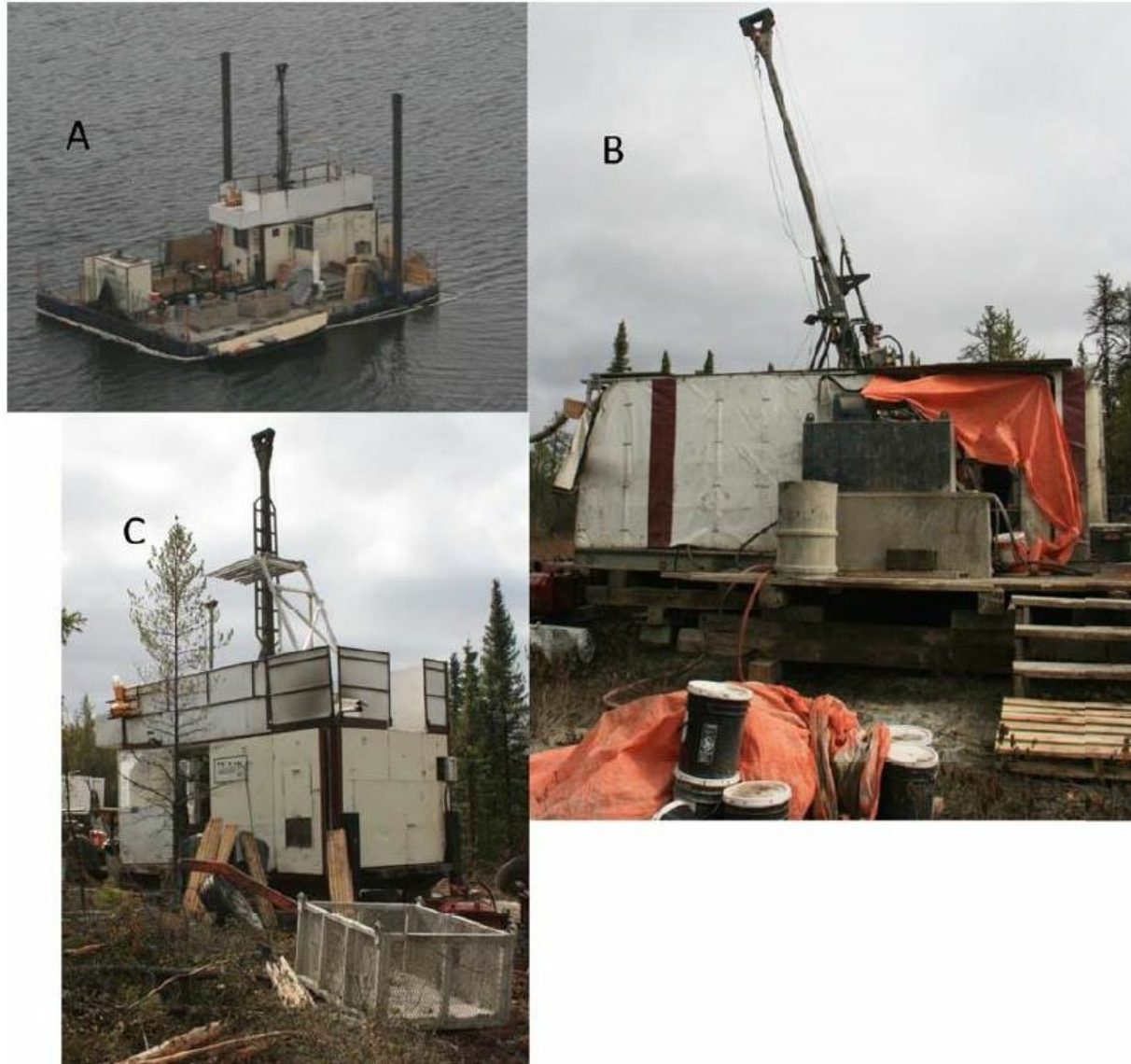
Figure 7-2: Drilling operations at the Project, A: Barge Mounted A5 Drill, B: Helicopter Transported A5 Drill, C: Skid Mounted A5 Drill
