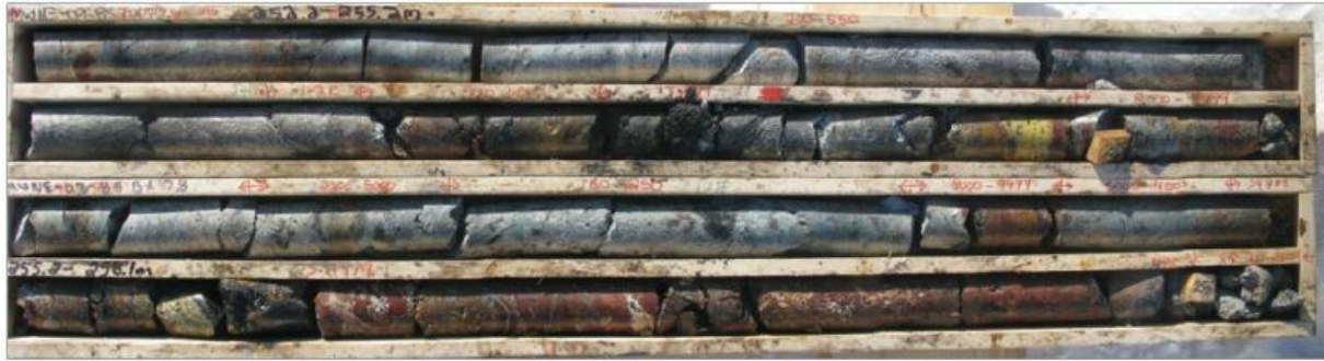
Figure 6-5: Uranium mineralized drill core from MWNE-085 from 252.2 m to 258.1 m
